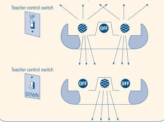
All these features add up to a system that is energy-efficient, easy to maintain, and provides a rapid payback (see **Table 2**). The base system costs less to install than a conventional lighting system with parabolic troffers and is projected to cut energy use by about 50 percent, providing an immediate payback. Field installations in 19 California classrooms have confirmed these savings.
