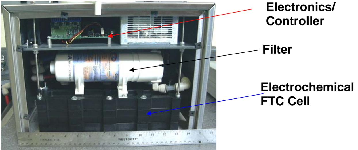
**Figure 1. Prototype system. System throughput is about 0.1 gallon per minute for tap water softening.**
