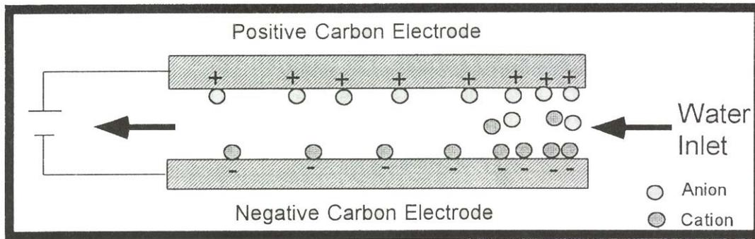
Figure 1: Illustrative Diagram of FTC with Charge Barriers
