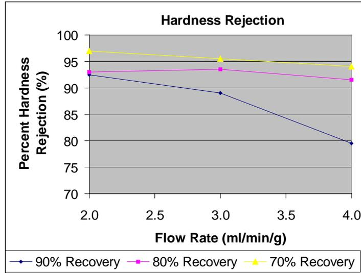
**Figure 2. Hardness rejection for the FTC.**
