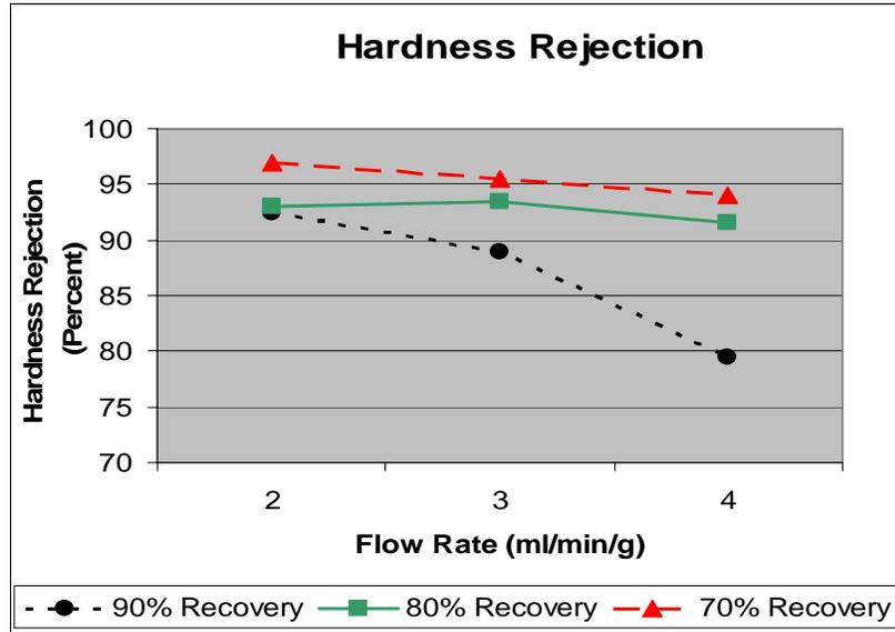
Figure 2: Hardness rejection for the FTC
