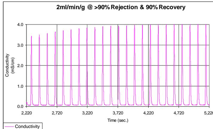
**Figure 3. High recovery repeatability data. Conductivity of outlet stream.**
