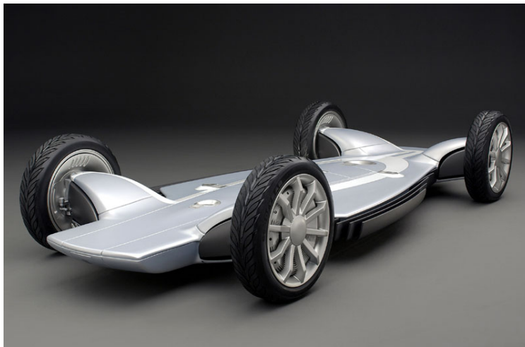
Figure 5-3: GM AUTOnomy Concept Skateboard Chassis 37
