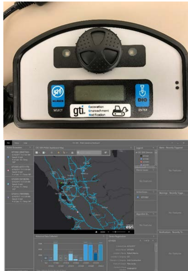
Figure 3: GPS Device on Excavator and Utility Monitoring Dashboard
