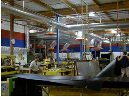
The manufacturing of solar heating panels used for pools
