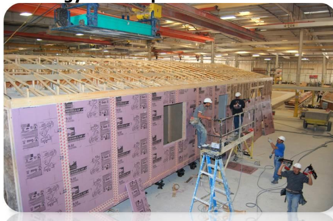
Figure 12: New Innovative Wall Insulation Leads to Less Energy Consumption for Manufactured Homes
