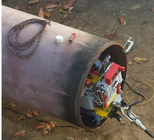
Figure 3: MS-EMAT Sensor Mounted on Pipeline Crawler
