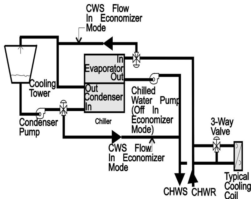
*This system does not meet the prescriptive requirement as it cannot operate in parallel with the chiller*
