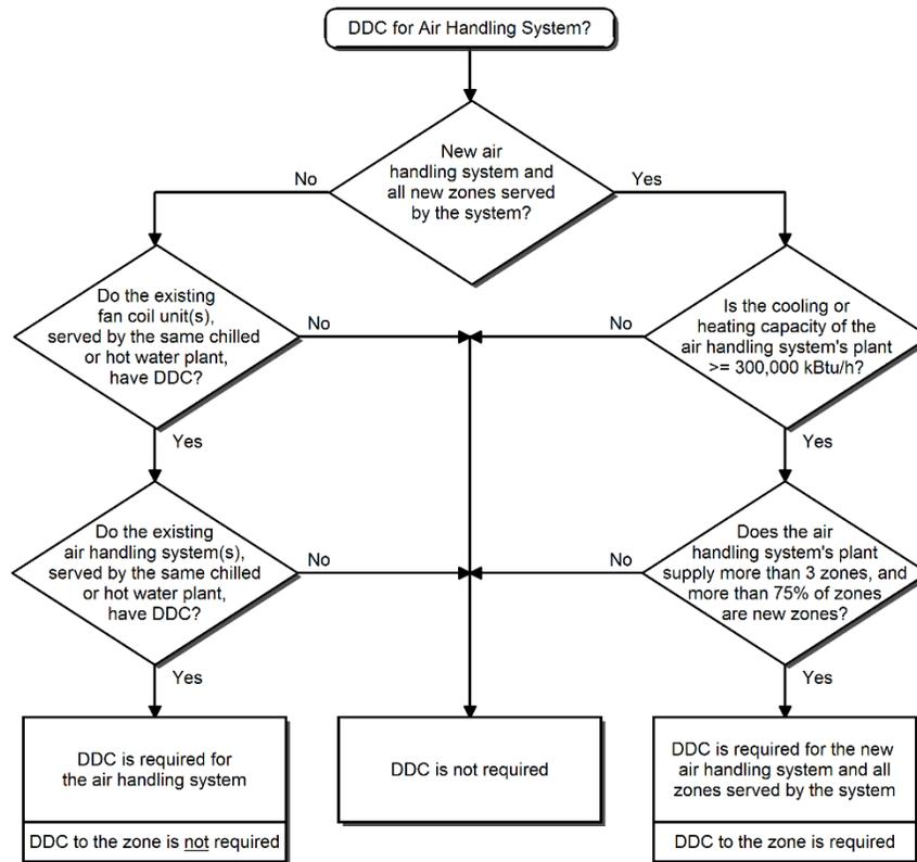
**Figure 4-18: Zone Terminal Unit Flowchart**
