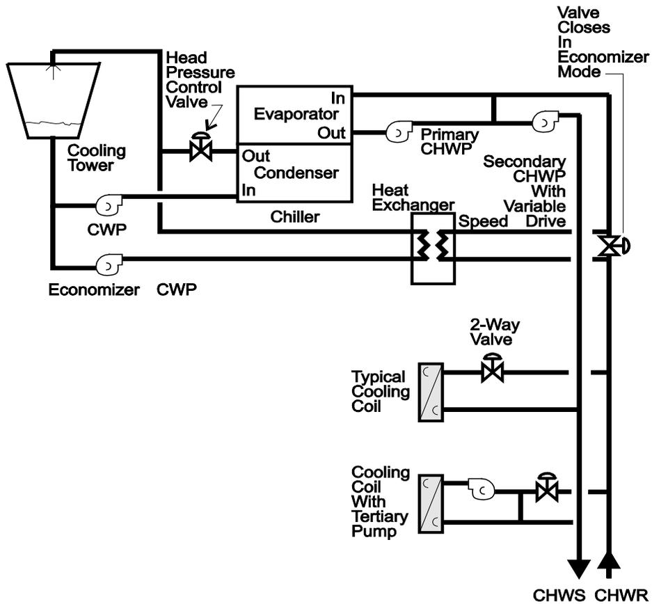
Figure 4-37: Air-Precooling Water Economizer
