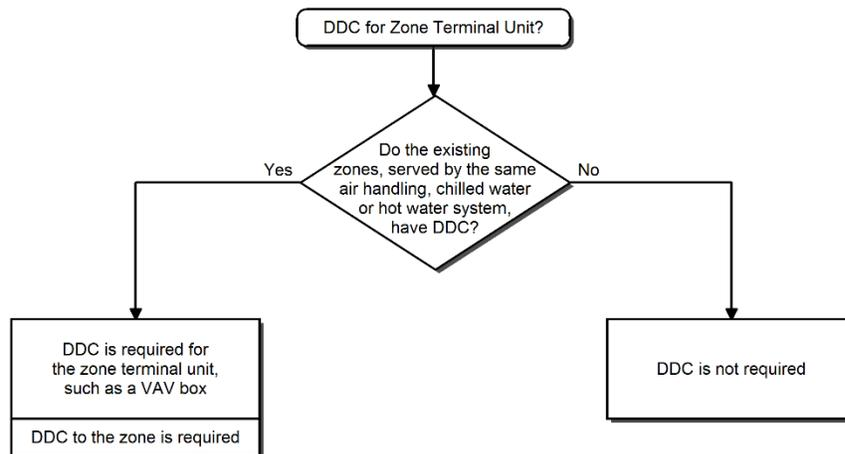
**Figure 4-19: Fan Coil Units Flowchart**
