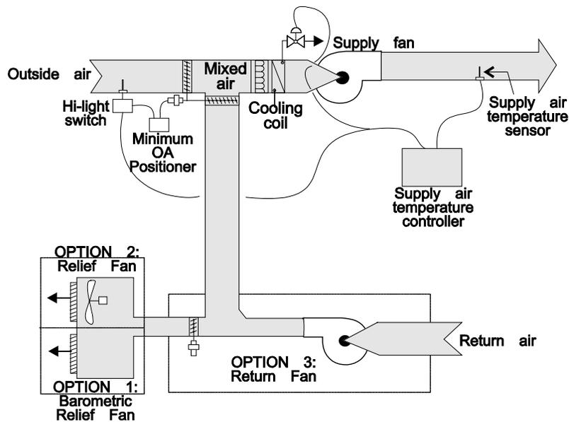
Figure 4-22: Typical Air-Side Economizer Control Sequencing
