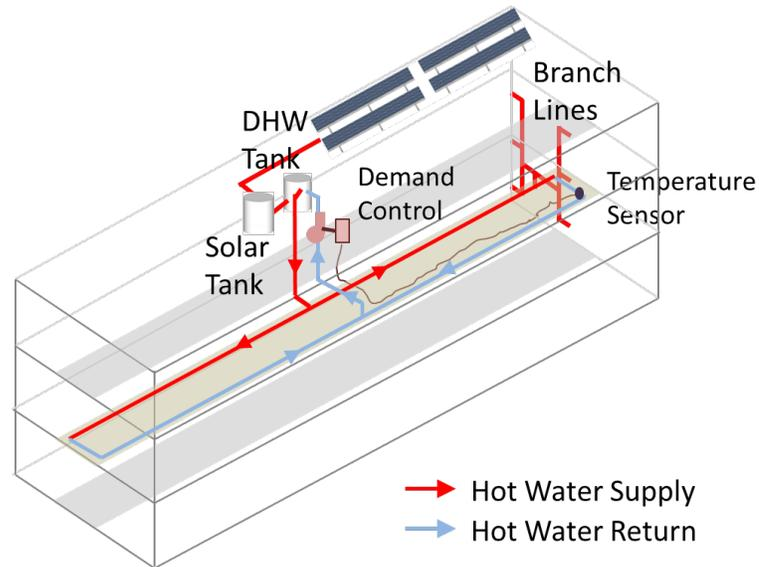
Figure 4-30 provides an example of how to implement dual-loop design in a low-rise multi-family building with a simple layout. In this example, the water heating equipment is located in the middle of top floor with each recirculation loop serving exactly half of the building. The recirculation loops are located in the middle floor to minimize branch pipe length to each of the dwelling units. The Figure 4-30 also illustrates how the solar water heating system and demand control are integrated.
