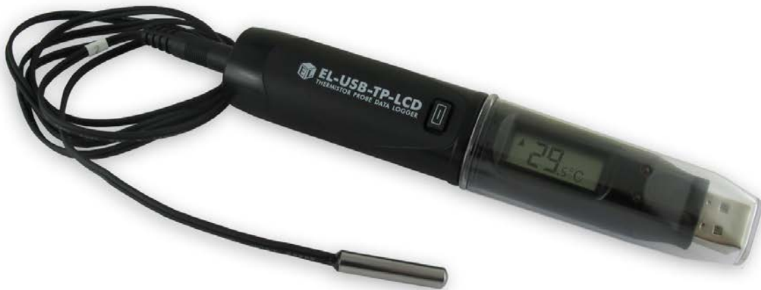
Figure 12. Temperature logger shown with stock thermistor probe. The detachable probe was replaced by a 4 m extension cable leading to the foil-wrapped bead thermistor shown in Figure 10.
