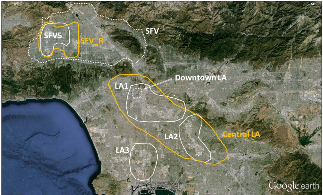
Figure 4. Boundaries of initial study areas LA1, LA2, LA3, and SFV5 (solid white lines) considered for meteorological modeling, installation of new stationary monitors, and mobile transects; LA1 and SFV5 were selected. Also shown are the boundaries of study areas Central LA and SFV_R (solid gold lines) used in analysis of personal weather station data, and the boundaries of the San Fernando Valley (SFV) and Downtown LA (dotted white lines).
