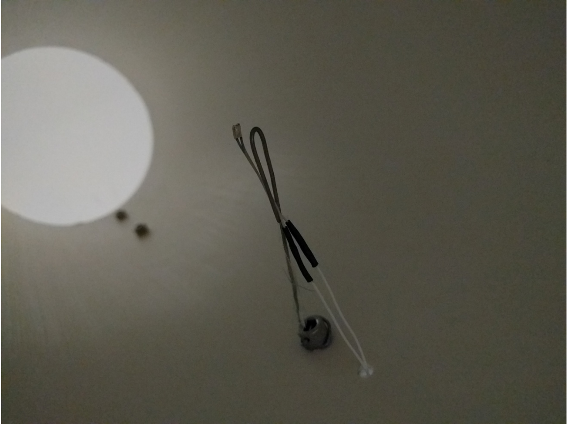
Figure 10. Bead thermistor wrapped in aluminum foil, then secured with clip in center of shield.
