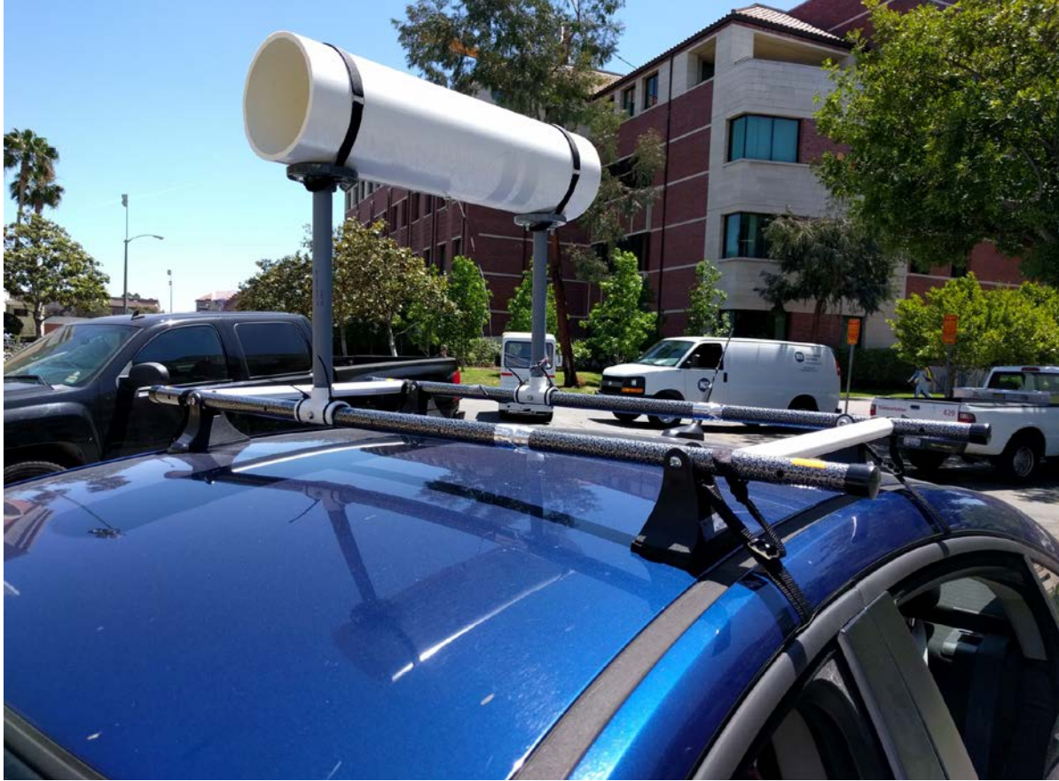
Figure 11. Shield on quick-install mount, strapped to the roof of a car, including white PVC-pipe shield, gray PVC-pipe vertical risers, aluminum tube roof mounting on plastic and rubber feet, and white PVC-pipe crossbeams. Straps with hooks (not shown) secure the bars to the vehicle frame.
