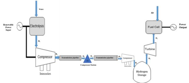
Figure D-2: Schematic of the Hydrogen Energy Storage System
