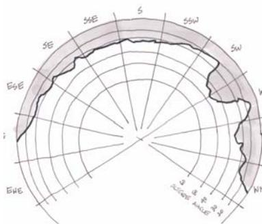
(a) This diagram shows the 22.5° compass segments used by the PV Calculator and the altitude angles.
