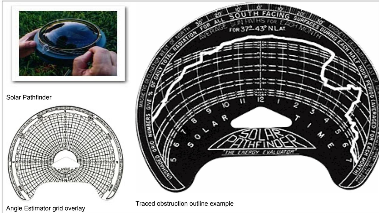
Figure 6 – Example Solar Access and Shading Analysis Instrument
