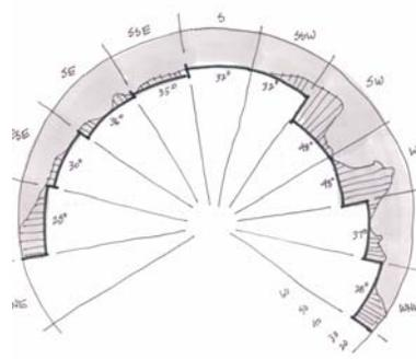
(b) Within each compass segment, the highest altitude is selected and used for that entire segment. This data is input into the PV Calculator.
