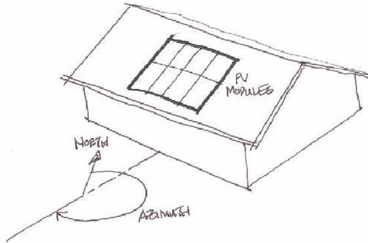
Figure 2 – Azimuth of the PV Array
