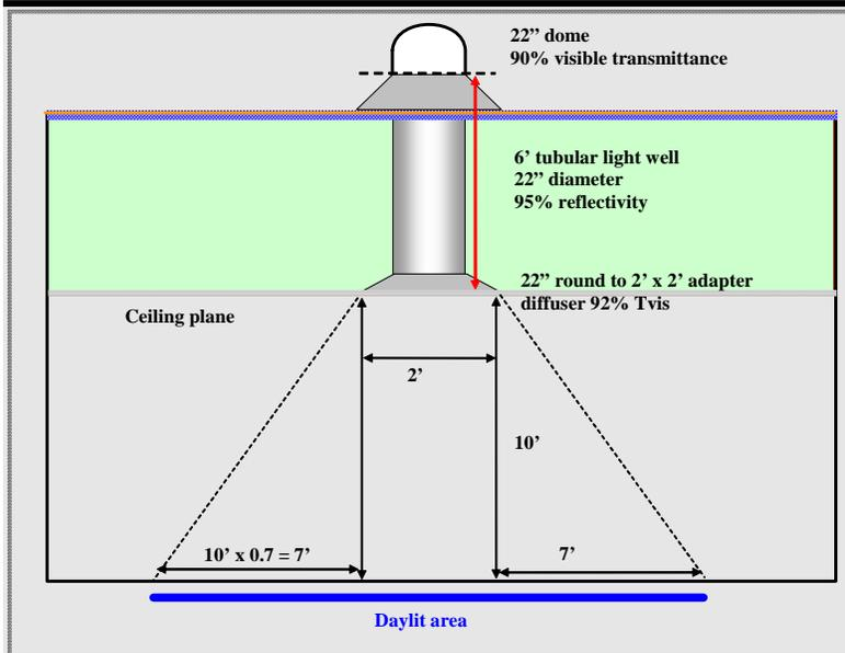
*Elevation Plan of Tubular Skylight*
