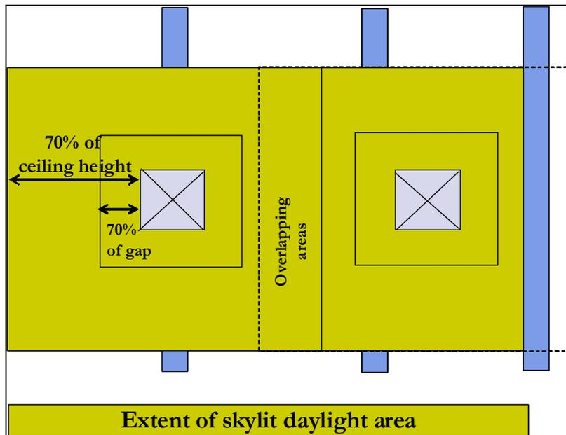
Figure 5-10 – Plan View of Daylit Area under Skylight with partitions
