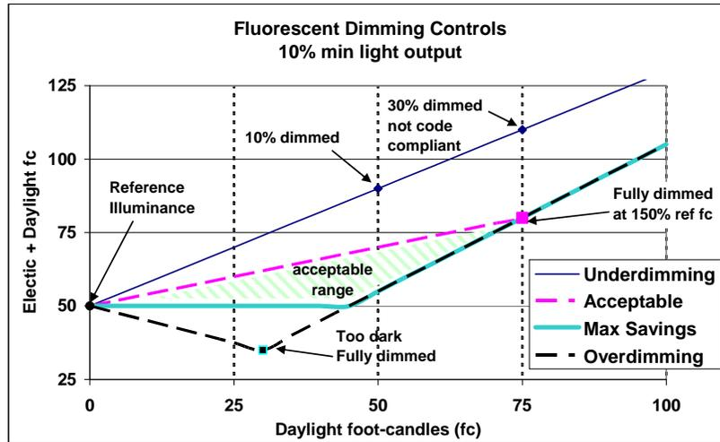
Figure 5-17 – Performance of dimming controls - total light (daylight + electric light) versus daylight
