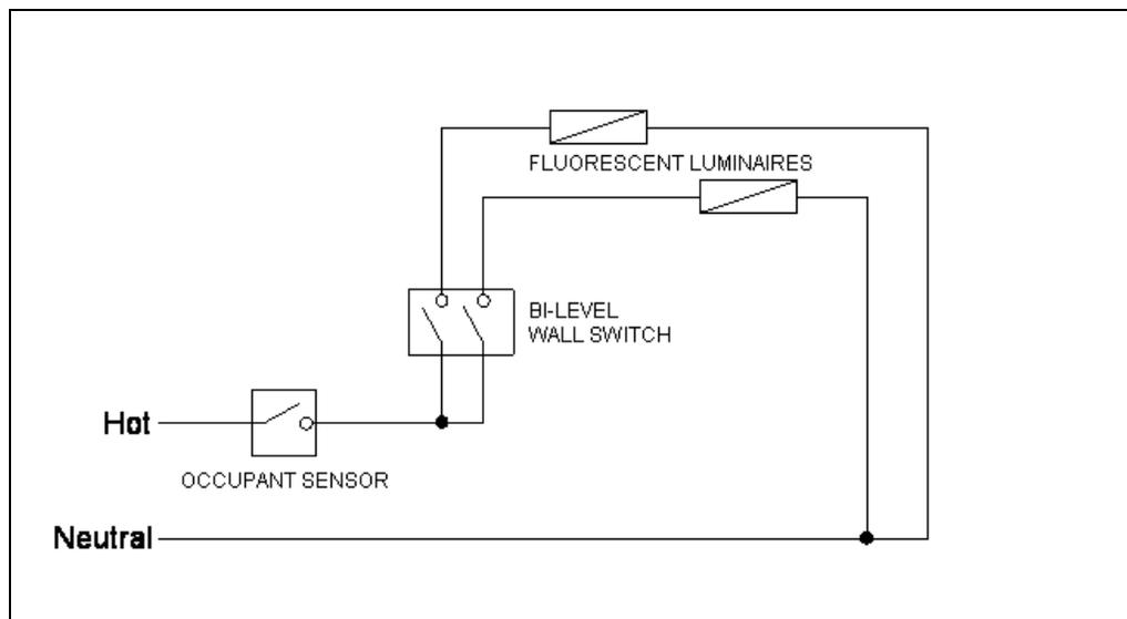
*Figure 5-19 – Occupancy Sensor with Manual Multi-level Switches*
