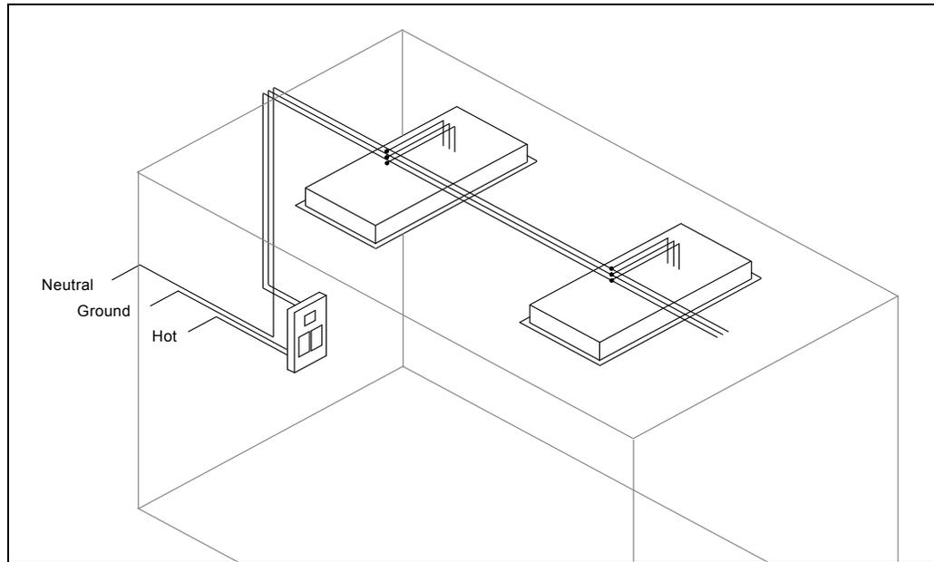
Figure 5-21 – Occupant Sensors with Multi-Level Control: “Inboard/Outboard” Approach
