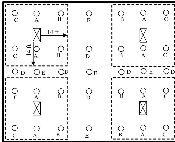
Figure 5-12– Lighting Plan Showing Daylit Areas and Circuits (20 ft ceiling height)
