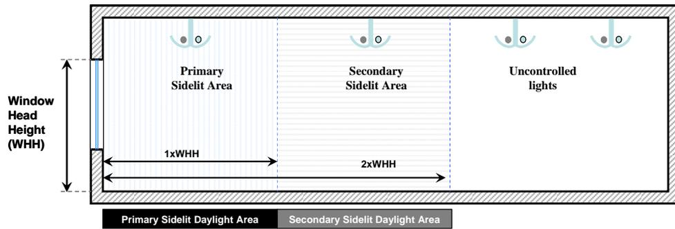
Figure 5-7 – Section view: Primary and secondary sidelit daylight area
