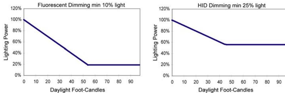
Figure 5-14 – Fluorescent and HID Power Draw in Response to Daylight
