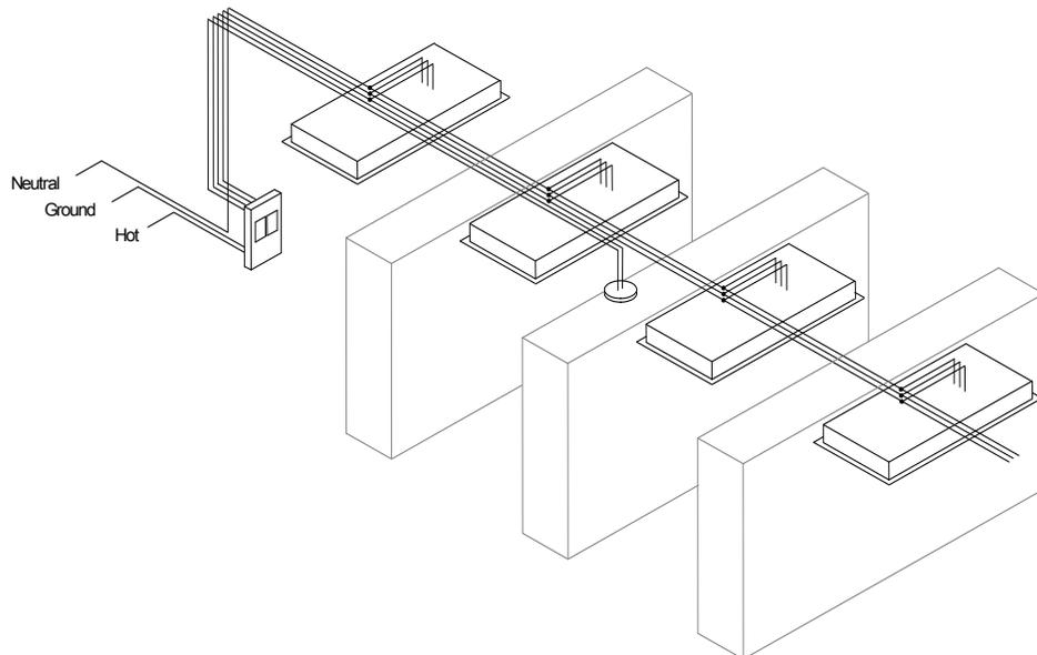
*Figure 5-23 – Photocell Dimming*
