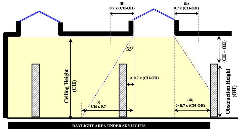
Figure 5-9 – Elevation View of Daylit Area under Skylight with partitions
