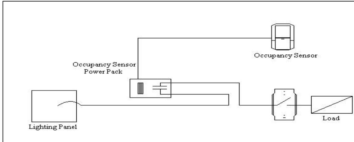
Figure 5-20 – Electrically Held, Normally Open, Latching Wall Switch With Occupancy Sensor
