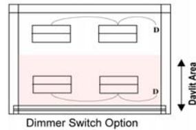
The Dimmer Switch Option controls the daylit and non-daylit areas separately, and the dimmer takes care of the multi-level illumination requirement.
