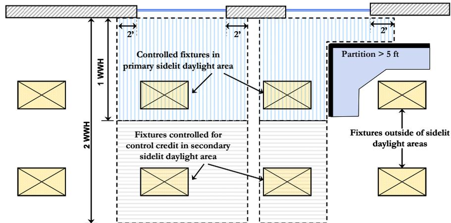
Figure 5-8 – Plan view of primary and secondary sidelit daylight area
