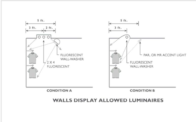
Per §146(c)3Bi, qualifying lighting must be mounted within 10 ft of the wall and appropriate wall lighting luminaires. (Luminaires with asymmetric distribution toward the wall or adjustable – directed toward the wall)
