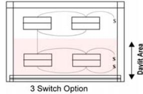
The 3 Switch Option also meets the requirements because switch "1" controls at least 50 percent of the lighting in the daylit area. Switch "2" controls the remainder of the lights in the daylit area and half of the lights in the non-daylit area. Switch "3" controls the remainder of lights in the non-daylit area.
