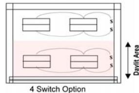
With the 4 Switch Option, the multi-level switching is provided separately to the daylit area and to the non-daylit area.
