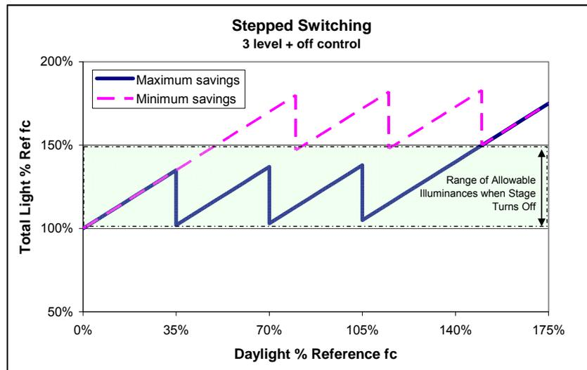
Figure 5-16 – Performance of compliant switching controls - total light (daylight + electric light) versus daylight
