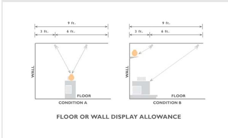
Per §146(c)3Bi & ii, wall display luminaires must be within 10 ft of the wall and directional and floor displays must be at least two feet away from the wall and also directional. Using these criteria, the allocations for the two conditions shown are as follows:
