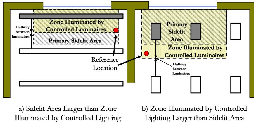
Figure 5-15 – Zone Illuminated by Controlled Luminaires and Reference Location for Measuring Reference Illuminance
