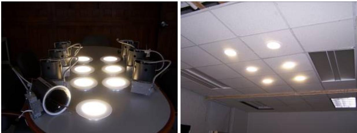
**Figure 7. The seven SPE-based LED downlight prototypes on a table (left), and six of them installed in an open area lab at the Lighting Research Center (right).**
