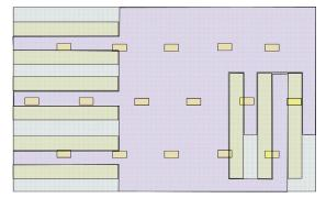
b)Skylit daylit zone (§130.1(d)) for controlling luminaires is limited by racks blocking daylight
