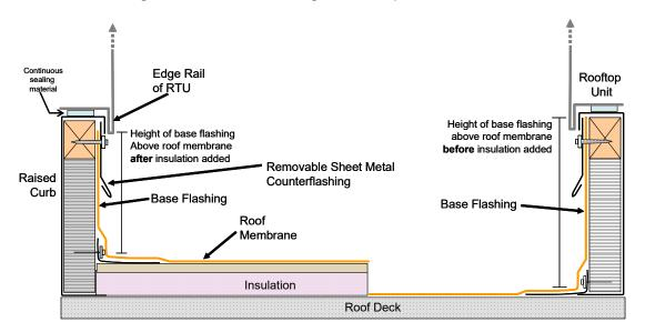
Figure 3-26: Base Flashing on Rooftop Unit Curb Detail
