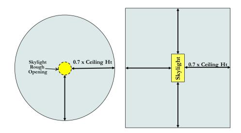
The shape of the skylit daylit zone will be similar in shape to the rough opening of the skylight, as shown in Figure 3-21.
