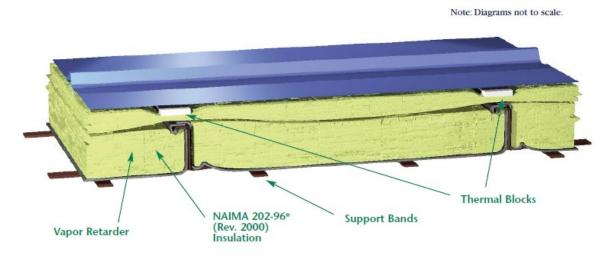
Figure 3-3A – Filled Cavity Insulation for Metal Building Roofs
