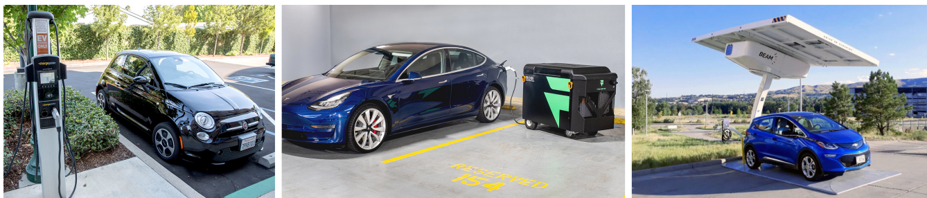
Figure 23: Examples of Different Charger Form Factors Based on the Local Environment
