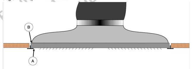
3. This must be a true statement (or not applicable) for the system to comply. Cloth back rubber adhesive duct tape (old style duct tape) does not meet the UL181 requirements for any new connections and may not be used as the primary method of sealing a duct connection. It may be used in conjunction with UL181
