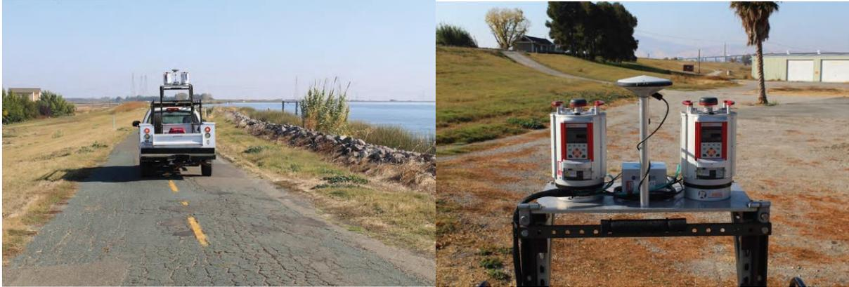
**Figure 4. Photos showing; A) the MLS (mobile laser scanning) truck operated by the USGS and employed for this study and B) the equipment rack showing dual laser scanners, IMU (inertial motion unit), and GNSS antenna.**
