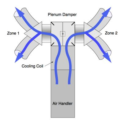
This diagram shows a common two-zone, single-damper system with both zones open (i.e., both zones are calling for cooling).
