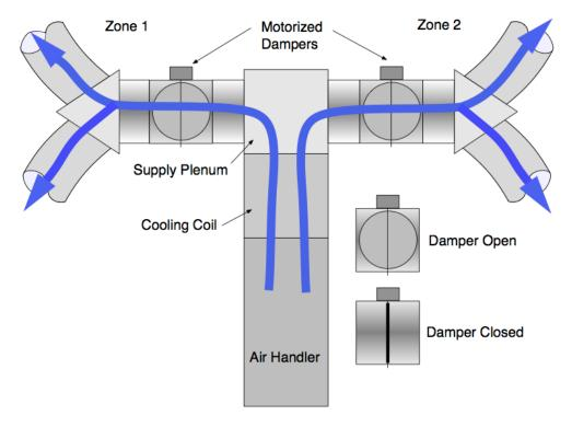
This diagram shows a common two-zone, two-damper system with both zones open (i.e., both zones are calling for cooling).
