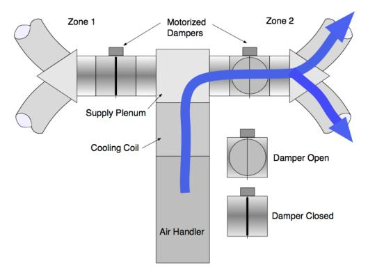
This diagram shows a common two-zone, two-damper system with zone 2 open (i.e., only zone 2 is calling for cooling).
