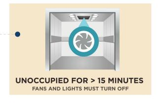
Controls must allow lighting and ventilation to remain operational in the event that the elevator cab is stuck when passengers are in the cab.
