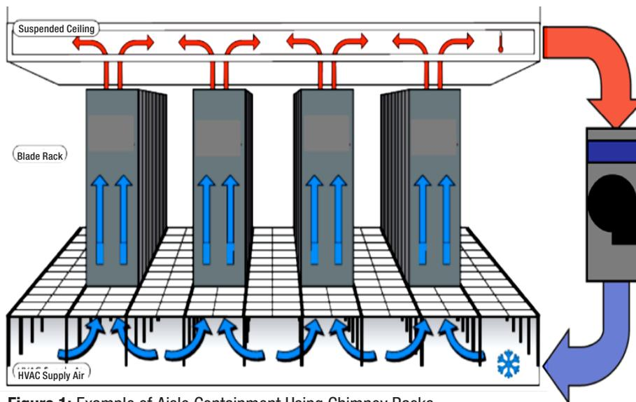
**Figure 1:** Example of Aisle Containment Using Chimney Racks
