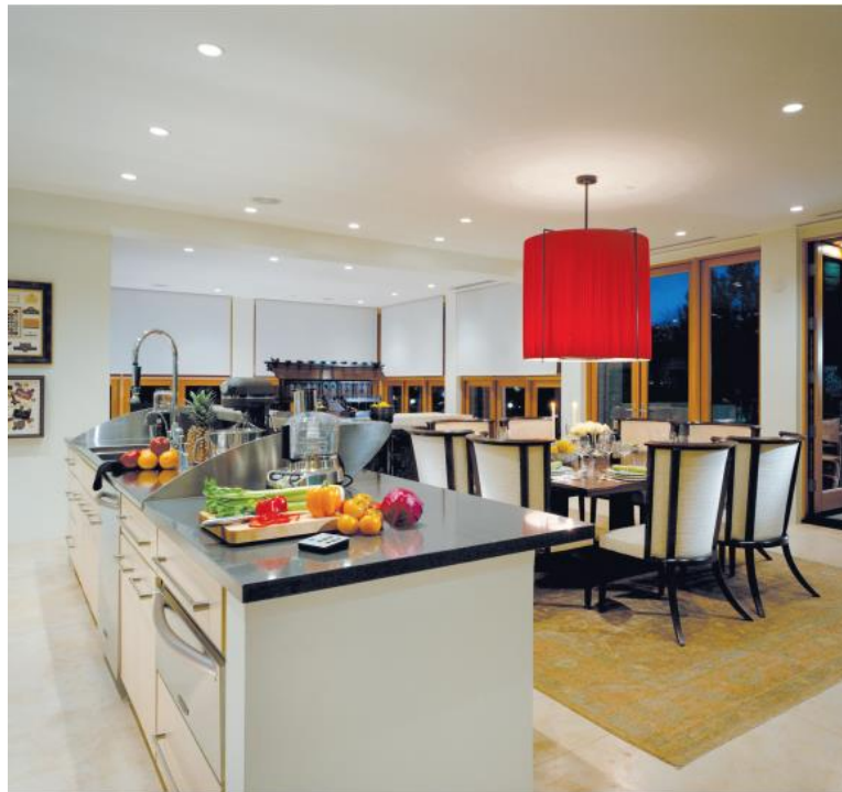
Figure 6-1 Recessed Downlight Luminaires in Ceiling
