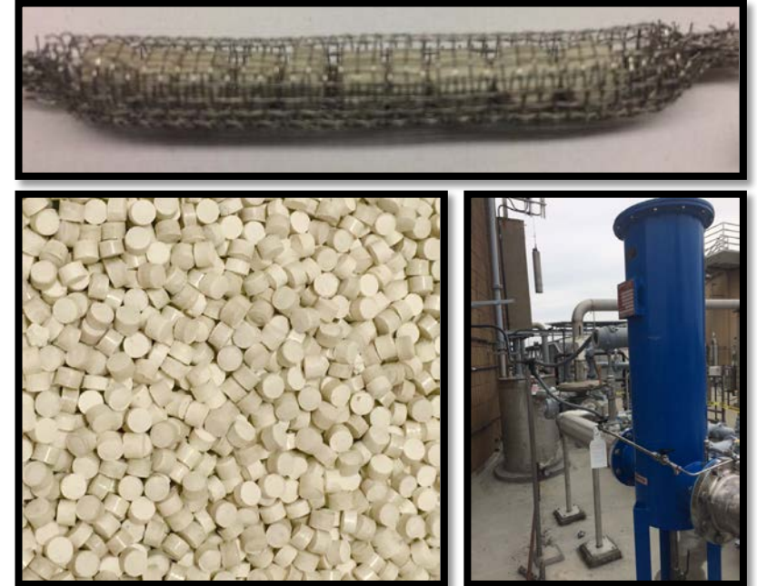
Sample of composite metal-organic framework pellets for exposure testing (top); tableted Gen-1 metal-organic framework adsorbent (bottom-left); Slipstream testing apparatus at the biogas site (bottom-right)
