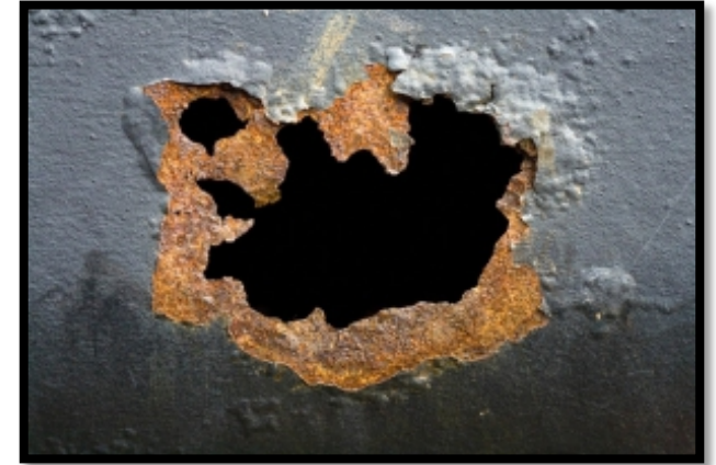
Photograph of corrosion damage to a pipeline. Source: https://blog.applus.com/wp-content/uploads/2016/04/corrosion-management-300x200.jpg
