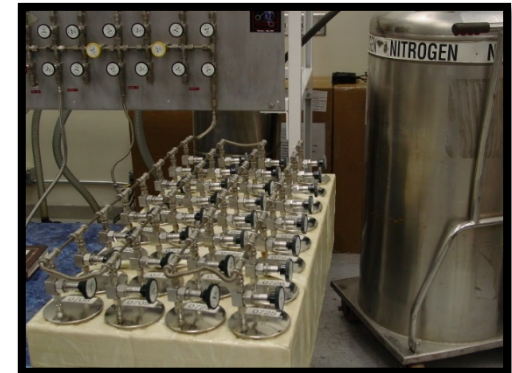
Figures: PG&E technician using a standardized procedure for sampling ( top ). Conditioned gas canisters await pressure testing ( bottom ).
