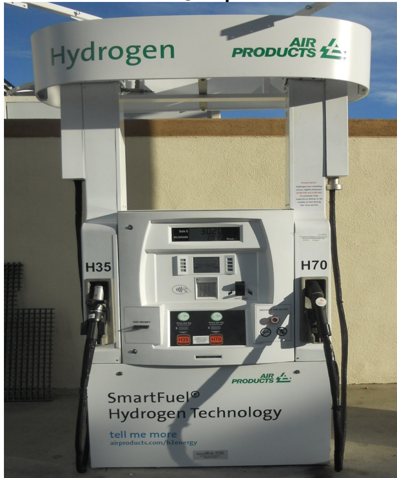
Figure 2: UC Irvine SmartFuel® Dispenser with DMS Certification
