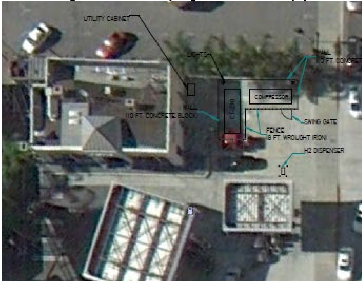
Figure 1: West Los Angeles SmartFuel® Hydrogen Station Initial Equipment Arrangement
