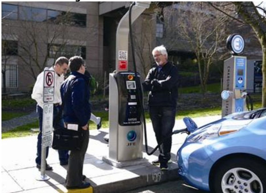
Figure 18: RAPIDAS / Kanematsu 208-volt Battery Backed Fast Charger on Portland's "Electric Avenue" 22
