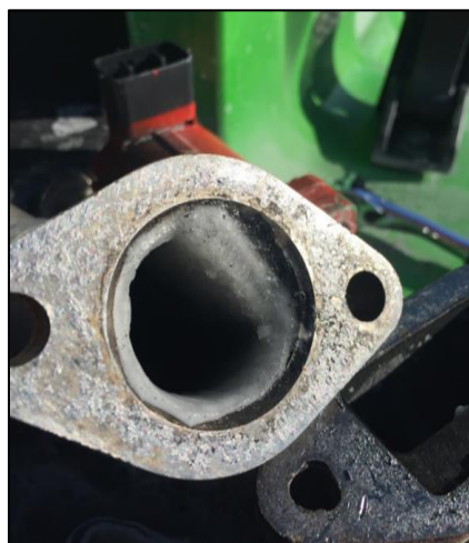
Figure A-16: Ice Formation in Exhaust Gas Recirculation Crossover Tube after Extended Idle in Minus 20 Degree Fahrenheit Conditions
