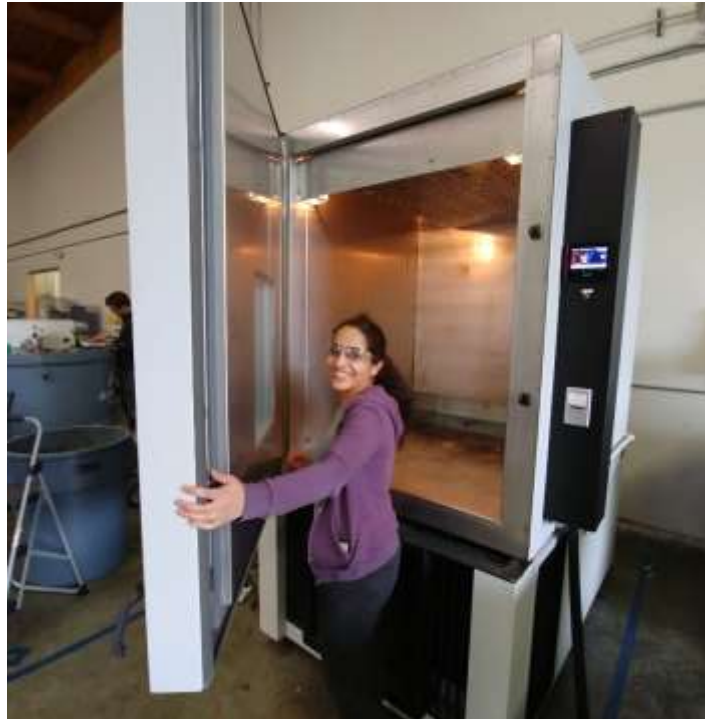
Figure 11: Environmental Test Chamber to Validate Temperature Requirements
