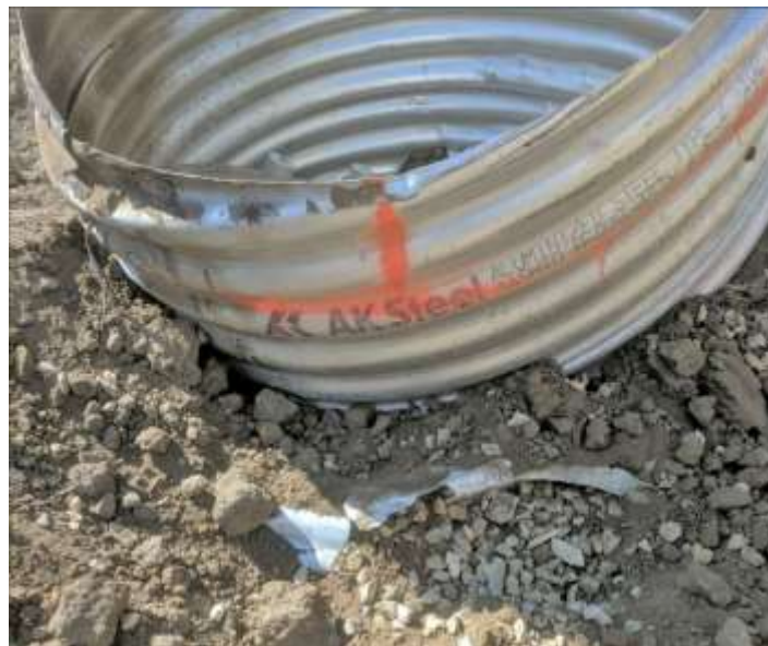
Figure 16: Vault Liner after Burst Test
