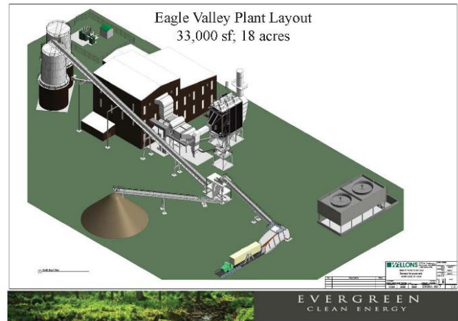
Figure ES-3: Footprint of 35 kW Electratherm Organic Rankine Cycle Generator Compared to 10 Megawatt Biomass Plant in Colorado
