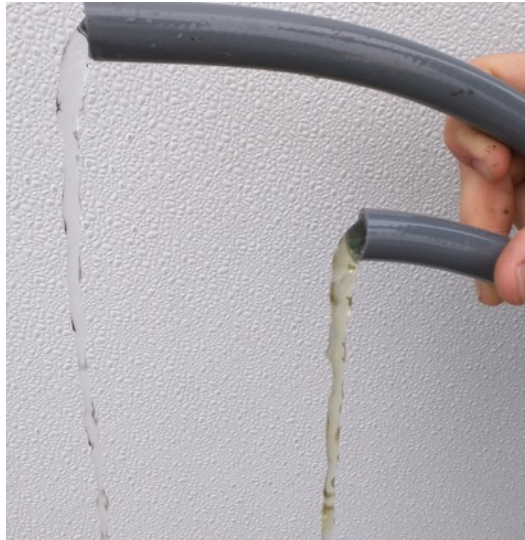
Figure ES-2: Water Purity Testing at Jackson Family Wines With (top) and Without (bottom) the PFO Recycler
