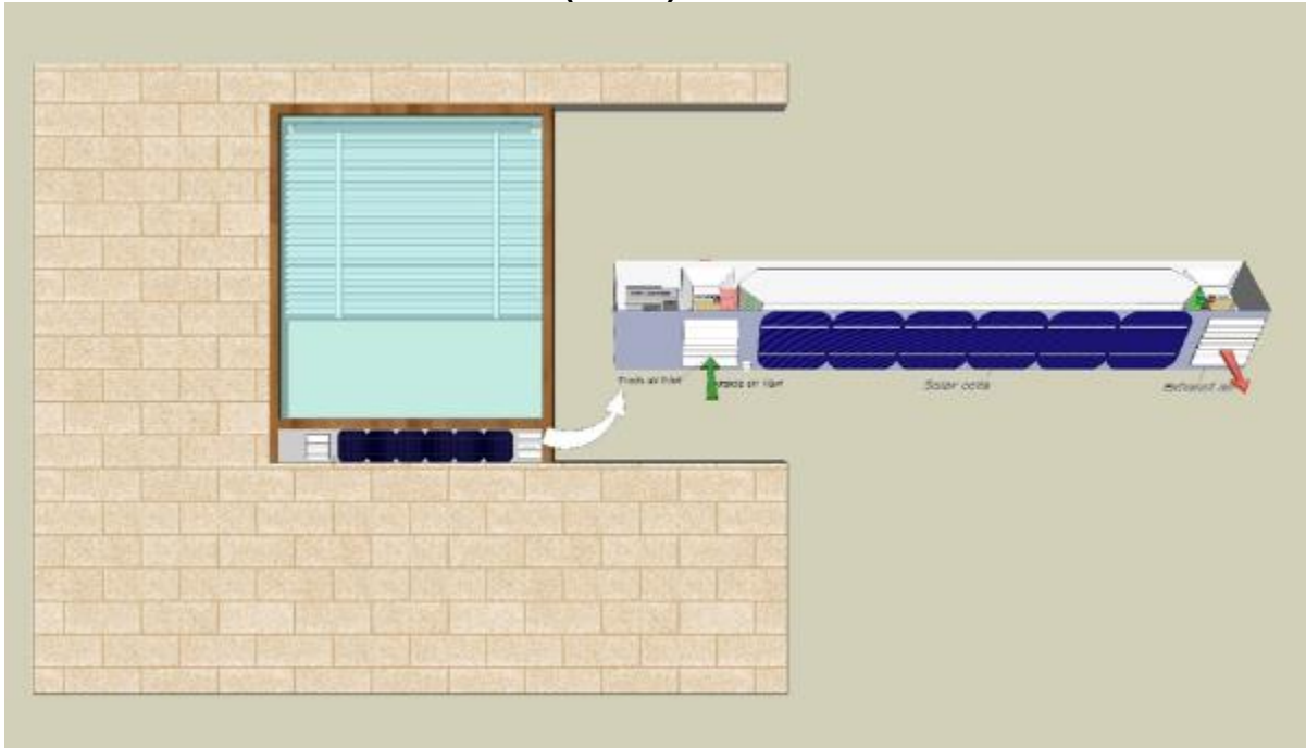
Figure 3.1: Illustration of a Packaged Local Ventilation and Energy Recovery (LVER) Unit
