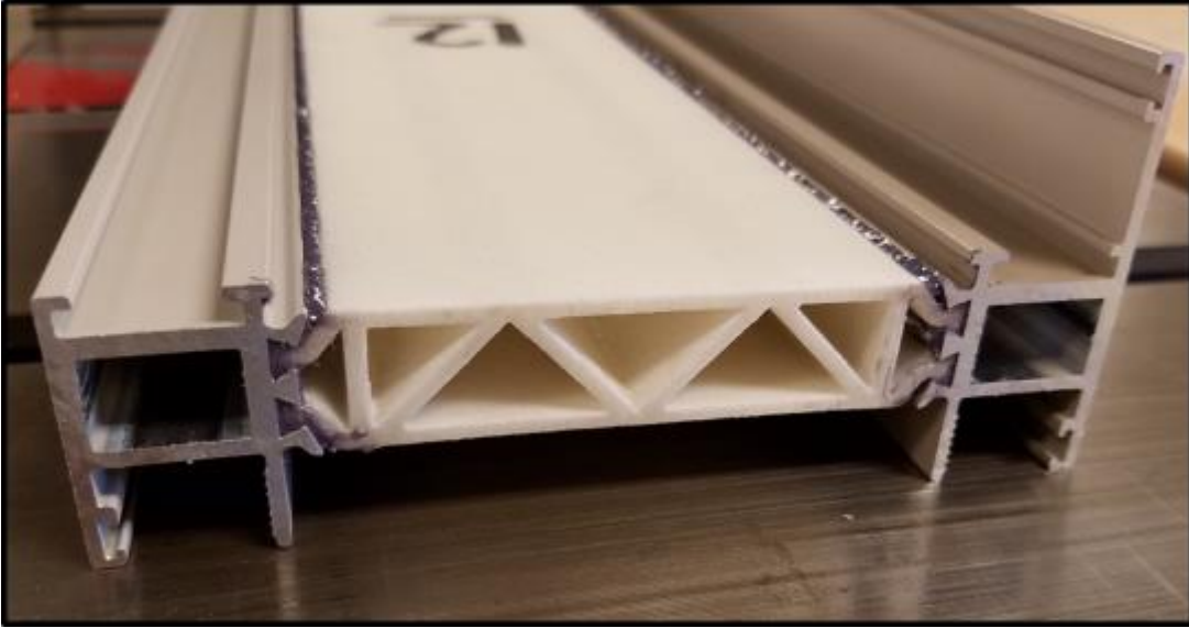
Figure 2.3: Image of the Assembled Prototype Truss Thermal Break Frame
