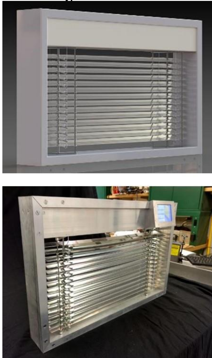
Prototype of variable-width blind assembly: computer rendering (top) and actual 432 x 711 millimeter (17 x 18 inch) prototype (bottom).
