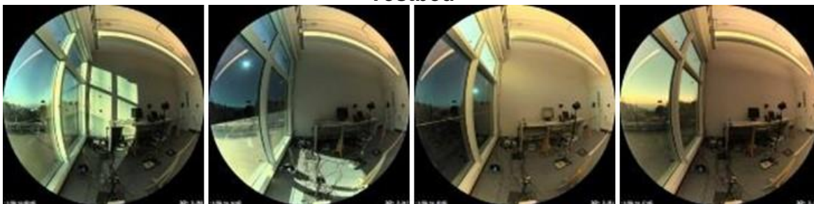
Figure 6.2: Three-Zone Electrochromic Window in the Advanced Windows Testbed
