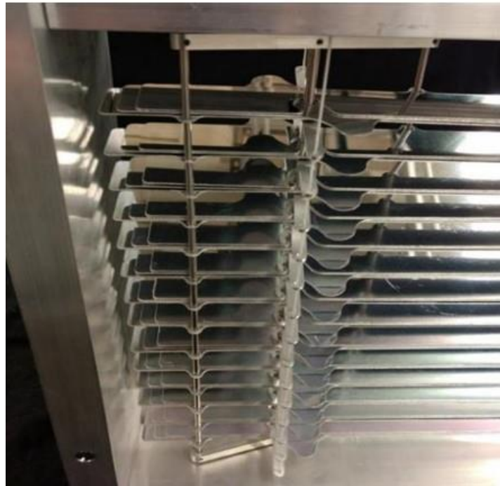
Stacked slats and a vertical rod actuation pivot: computer rendering (top) and actual prototype (bottom).
