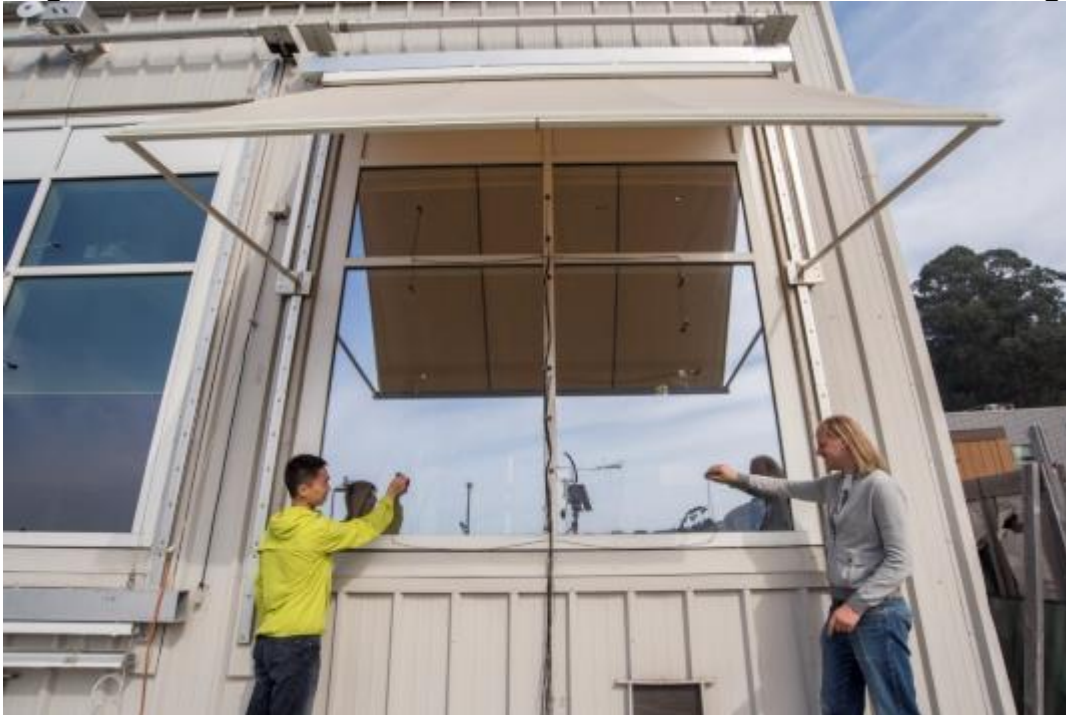
Figure 5.10: LBNL Advanced Windows Testbed with a Fabric Awning
