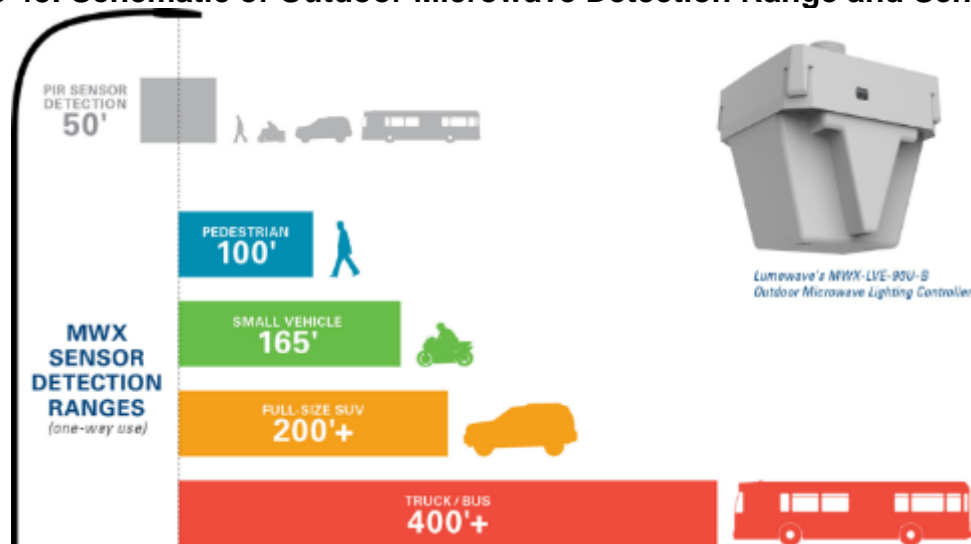
Figure 48: Schematic of Outdoor Microwave Detection Range and Sensitivity
