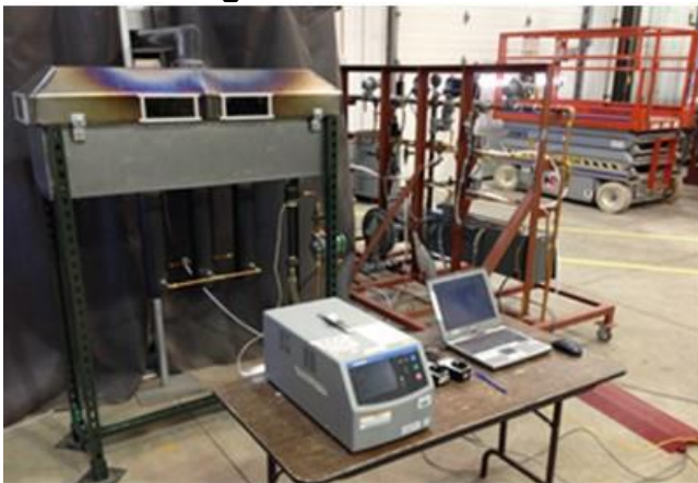
Figure 7: Lab-Scale Ribbon Burner Experimental Setup
