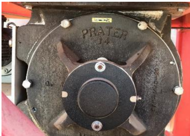
Dynamic vacuum air locks for product discharge
