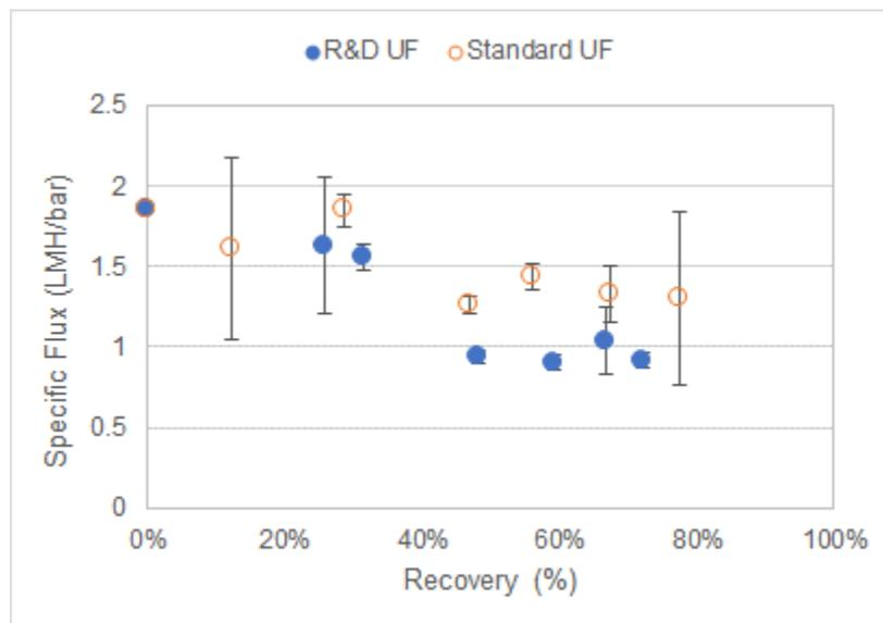
Conversion: 1 LMH/bar is equivalent to 0.04 GFD/psi.
