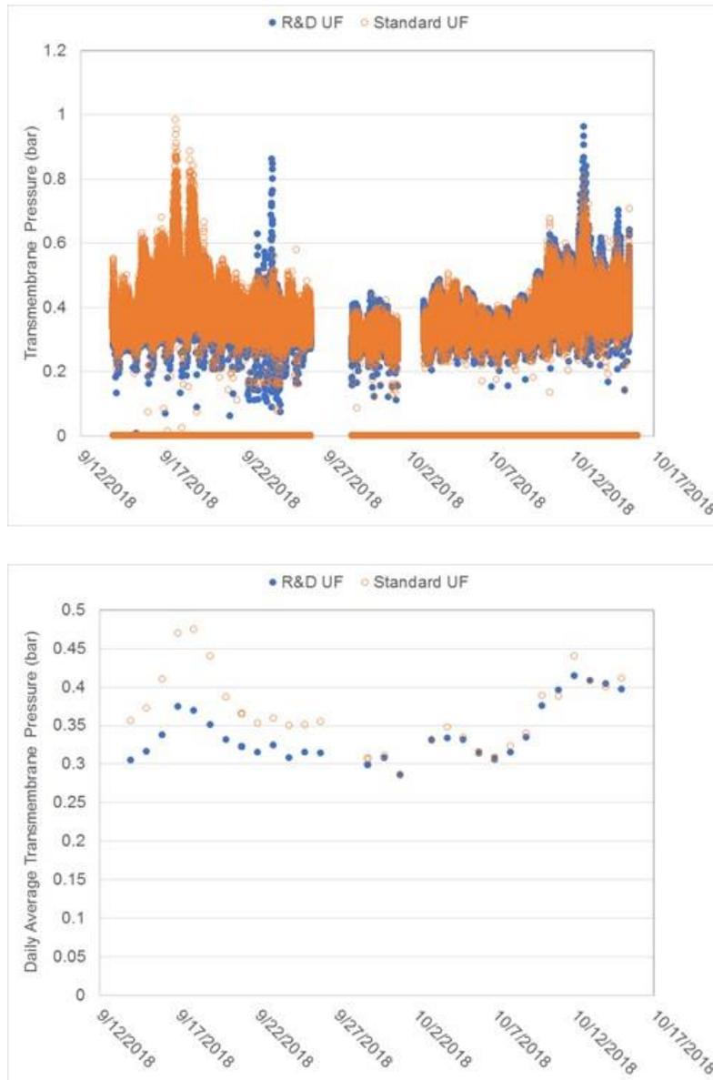
Transmembrane Pressure (upper panel) and Daily Average Transmembrane Pressure (lower panel) . Conversion: 1 bar is equivalent to 14.50377 psi.
