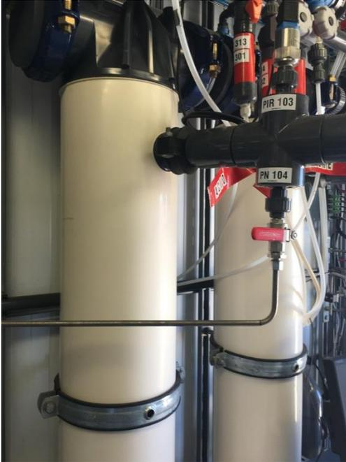
**Figure 2-3** Photo of R&D UF Membrane Module (foreground)
