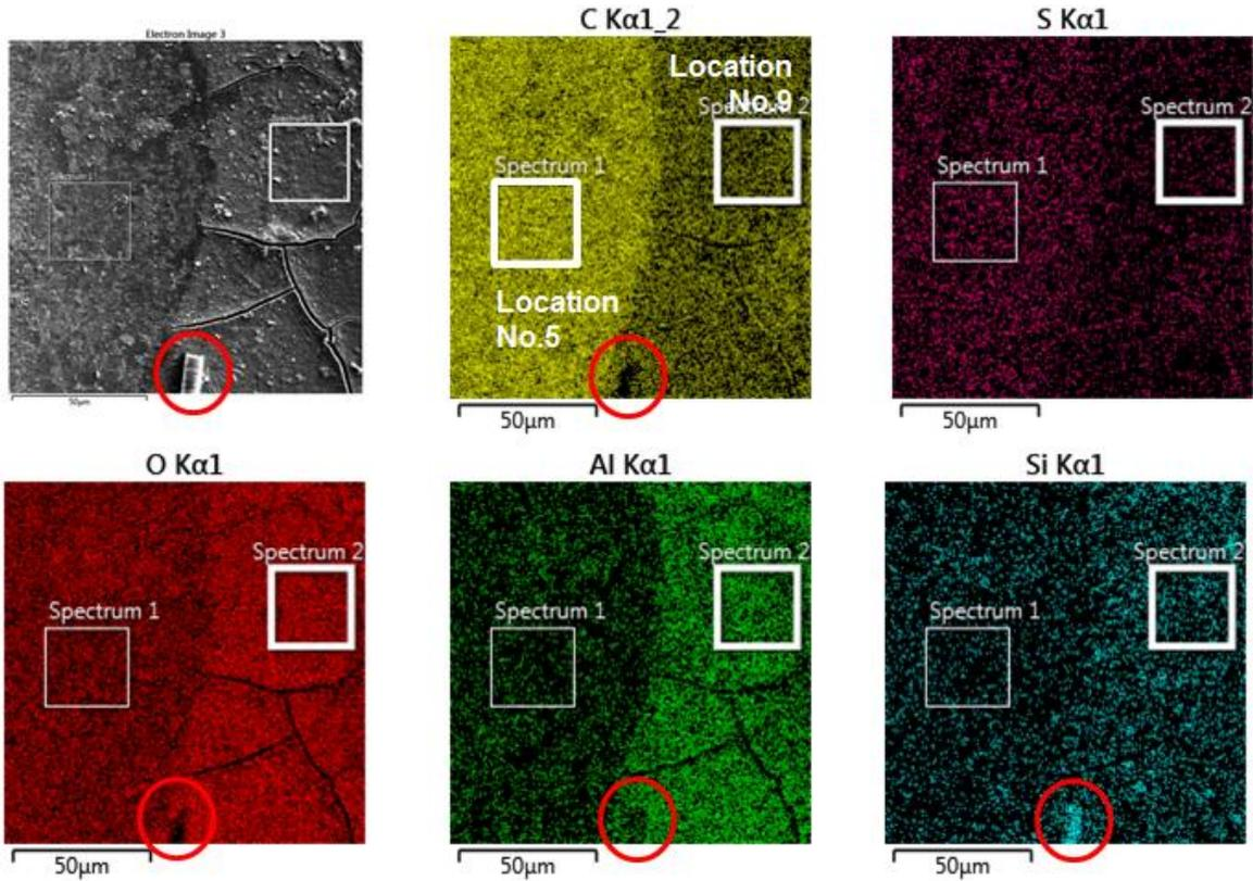
Images Clockwise from Upper Left: SEM Electron Image, Carbon Intensity, Sulfur Intensity, Silica Intensity, Aluminum Intensity, and Oxygen Intensity. Specific location of spectra collection locations No. 5 and No. 9 are highlighted in the Carbon Intensity image plate. Red circle refers to a silica crystal deposited on the membrane surface.
