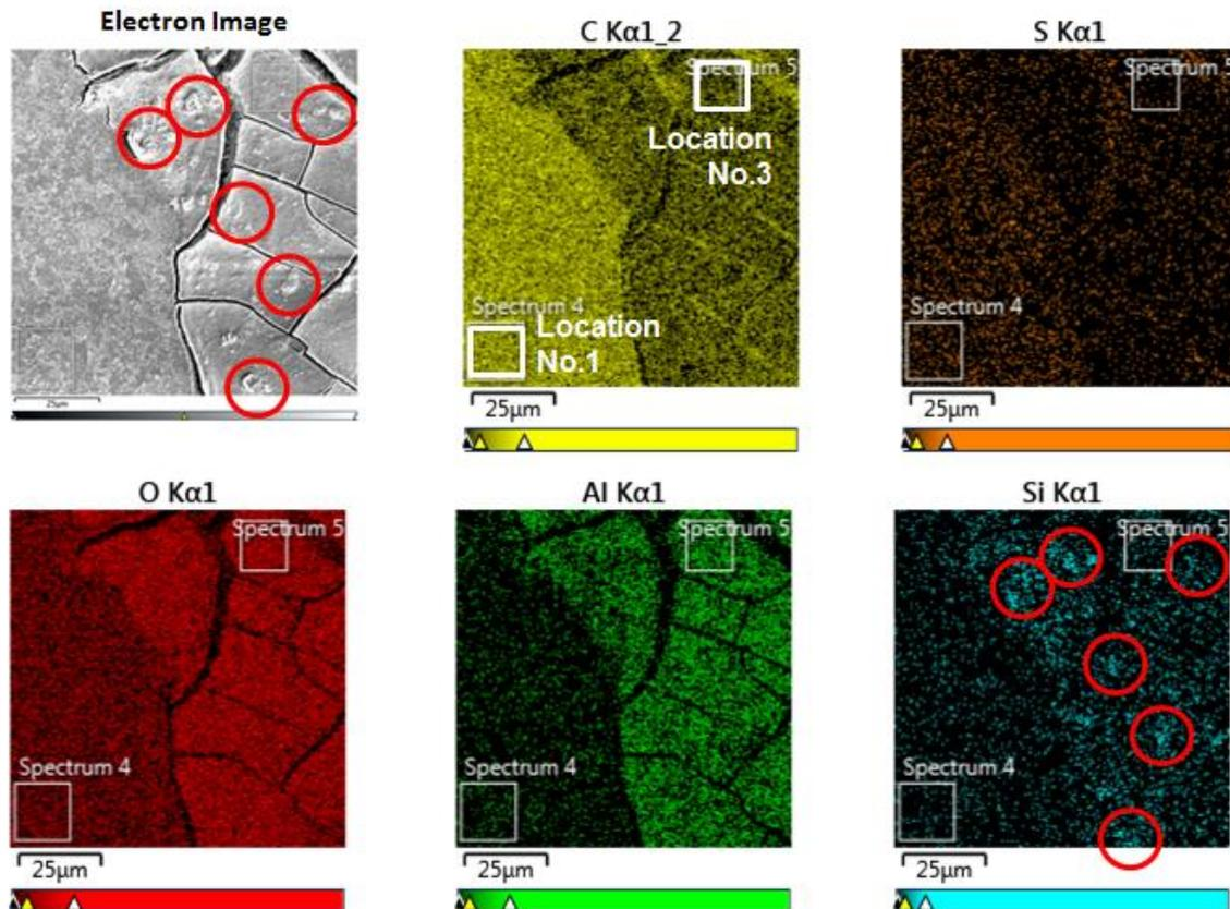
Images Clockwise from Upper Left: SEM Electron Image, Carbon Intensity, Sulfur Intensity, Silica Intensity, Aluminum Intensity, and Oxygen Intensity. Specific location of spectra collection locations No. 1 and No. 3 are highlighted in the Carbon Intensity image plate. Red circles highlight some examples of silica colloids deposited in the membrane surface, as discussed in the accompanying text.
