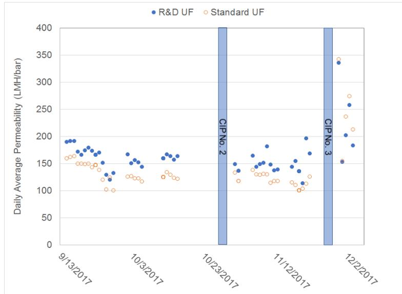
**Conversion: 1 LMH/bar is equivalent to 0.04 GFD/psi.**
