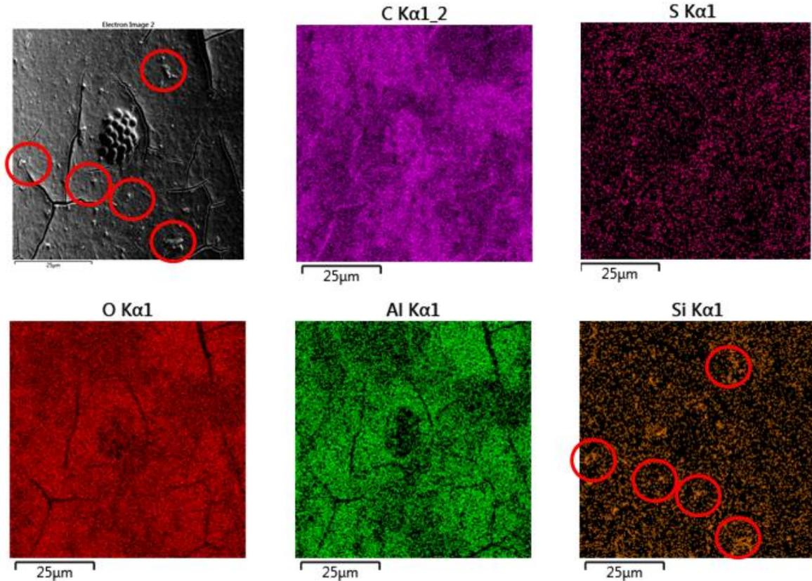
Images Clockwise from Upper Left: SEM Electron Image, Carbon Intensity, Sulfur Intensity, Silica Intensity, Aluminum Intensity, and Oxygen Intensity. Red circles highlight some examples of silica colloids deposited in the membrane surface.
