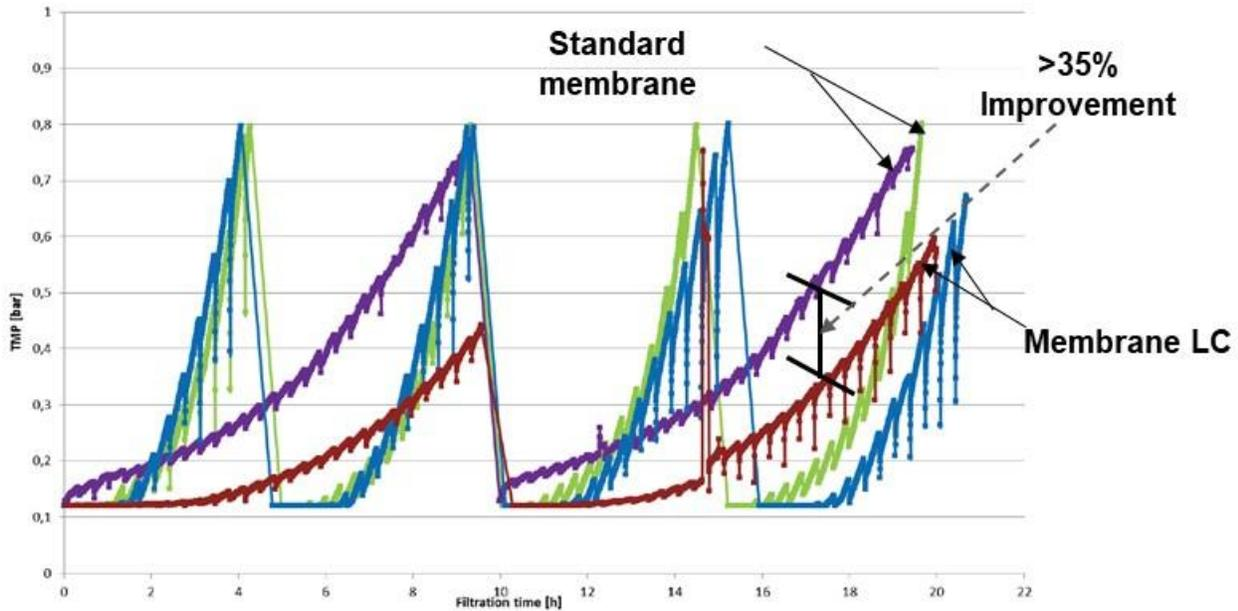
Tests were performed over a period of 20 hours, using standard PSU membrane chemistry at 75 L/m<sup>2</sup>-hr (green line) and 150 L/m<sup>2</sup>-hr (purple line) and Membrane LC (PSU-PEO-Polysiloxane) chemistry at 75 L/m<sup>2</sup>-hr (blue line) and 150 L/m<sup>2</sup>-hr (red line).
