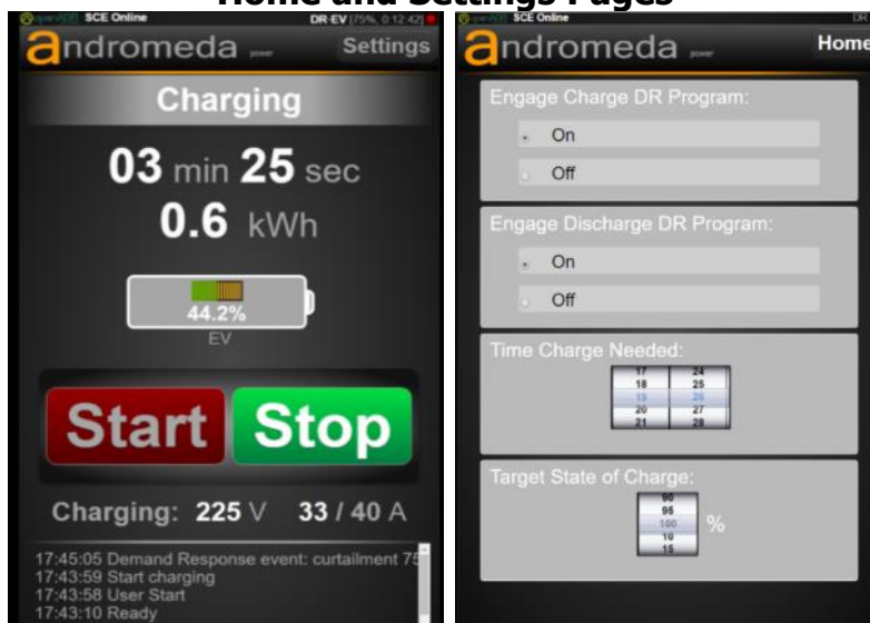
Figure 5: Screen Shots from Plug-In Electric Vehicle Mobile App: Home and Settings Pages
