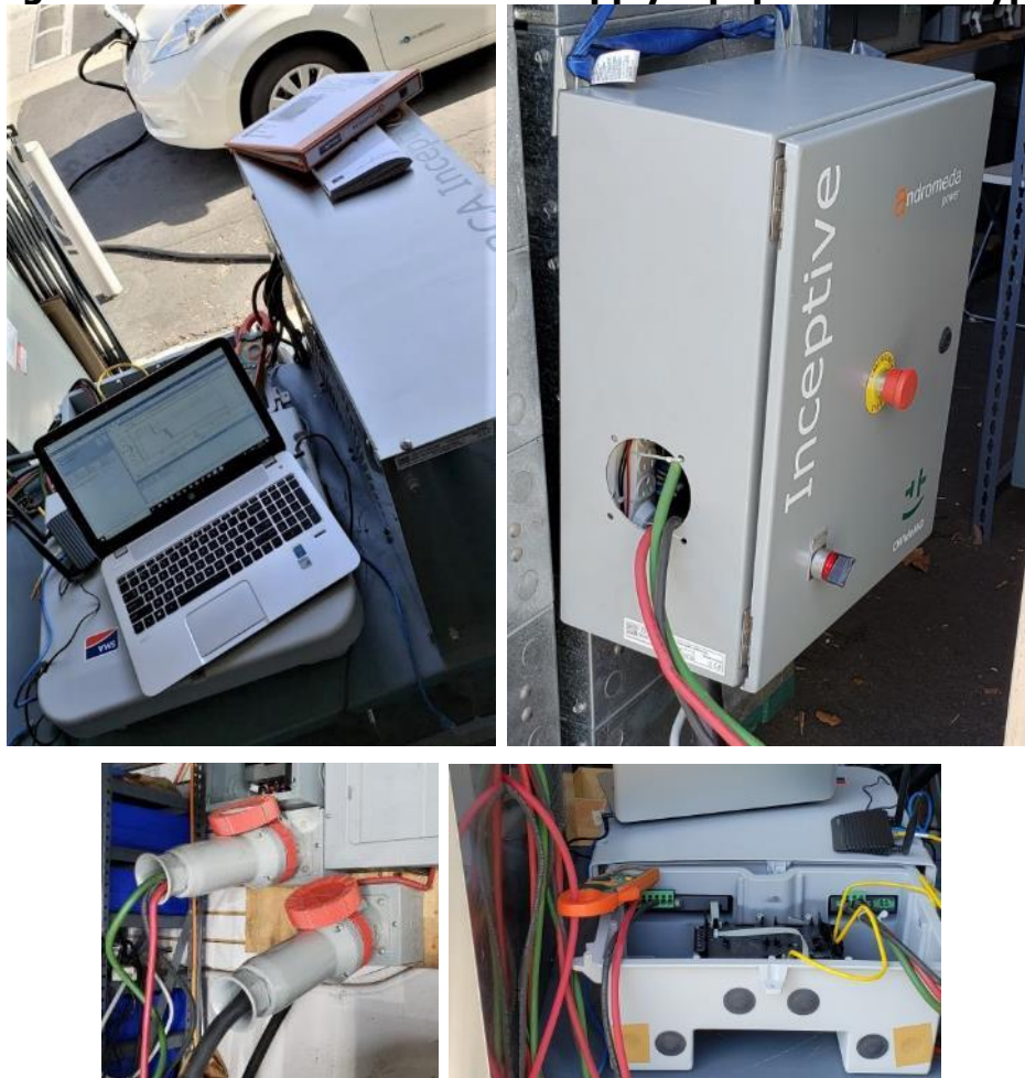
Figure 22: V2G Electric Vehicle Supply Equipment Prototype
