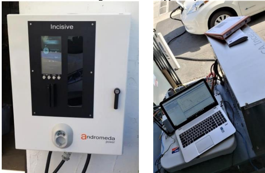
Figure 2: Vehicle-Grid Integration Prototype Capable of V1G and V2G
