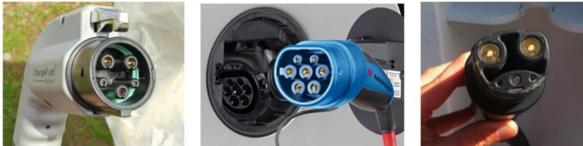
US Type 1 SAE (left), European Type 2 Mennekes (middle), and Tesla (right)
