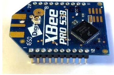
Figure 5: Programmable XBee-PRO 900HP, Model XBP9B-DMUTB002
