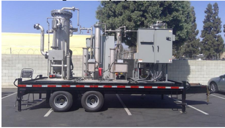
Figure 26: Three Stage Cleanup System Installed on 16' Trailer
