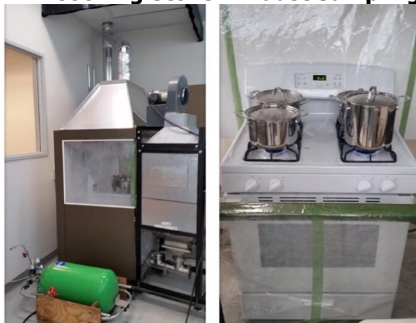
Figure 24: Cooking Stove Exhaust Sampling Setup
