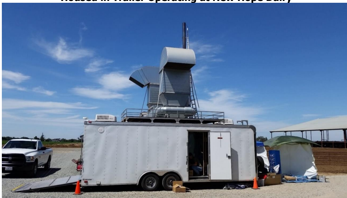
Figure 2: Transportable Photochemical Smog Chamber Housed in Trailer Operating at New Hope Dairy
