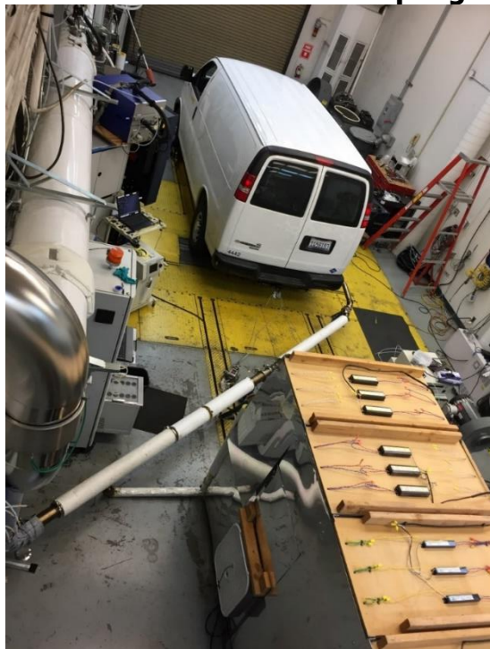
Figure 23: Vehicle Exhaust Sampling Setup
