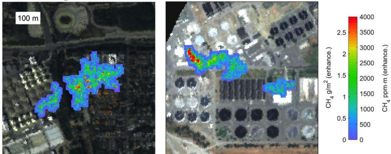
Examples of persistent methane point sources at a small number of wastewater treatment facilities. Left: Hyperion treatment plant, Right: Santa Clara/San Jose plant.
