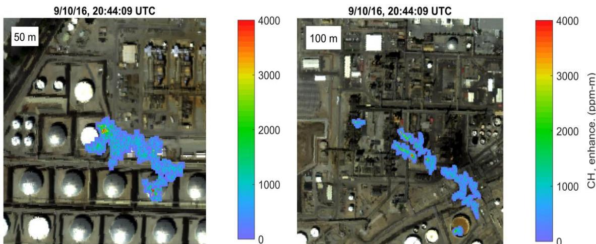
(Left) venting or leaking storage tanks, (Right) methane from combustion sources.
