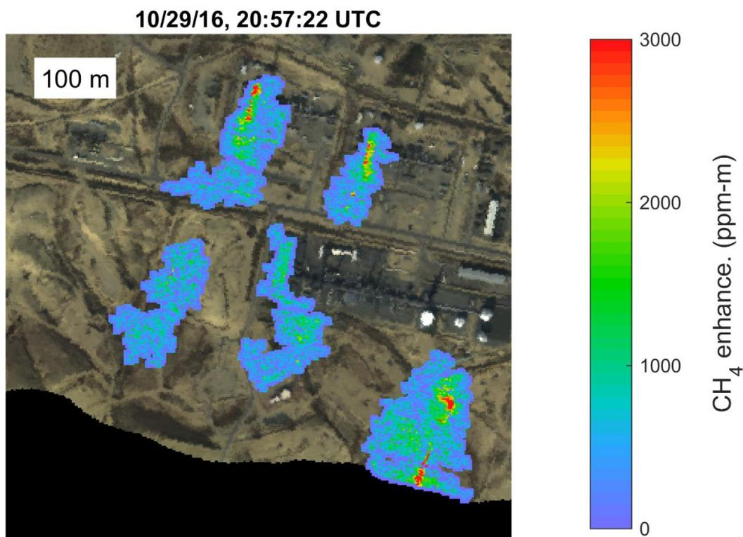
Gas processing facility in Elk Hills showing methane plumes from two of three large compressors (top) and one or more flaring stacks (bottom). These are all highly intermittent sources.
