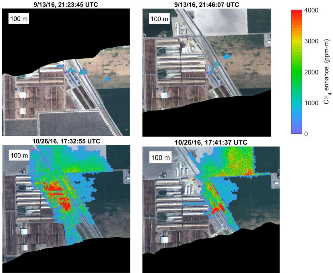
The difference in plume appearance between the two dates is attributed primarily to different wind speeds.
