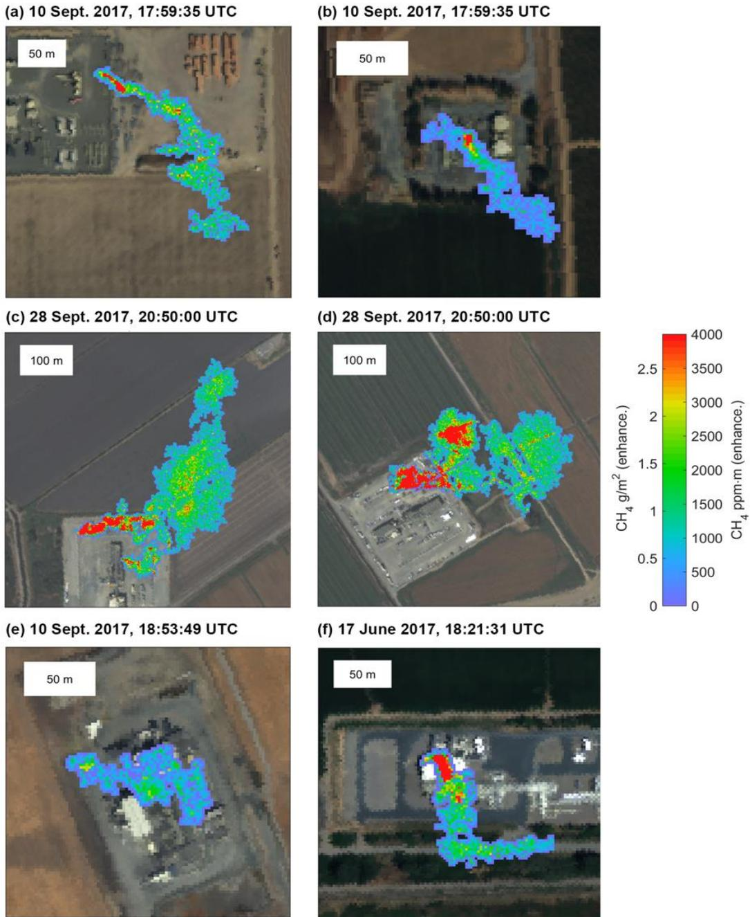
**(a) Gill Ranch venting from shutdown stack, (b) Lodi –likely dehydrator venting, (c) and (d) McDonald Island south and north platforms - venting from shutdown stacks and one compressor, (e) Kirby Hills – venting from shutdown stack, (f) Wild Goose compressor loss.**
