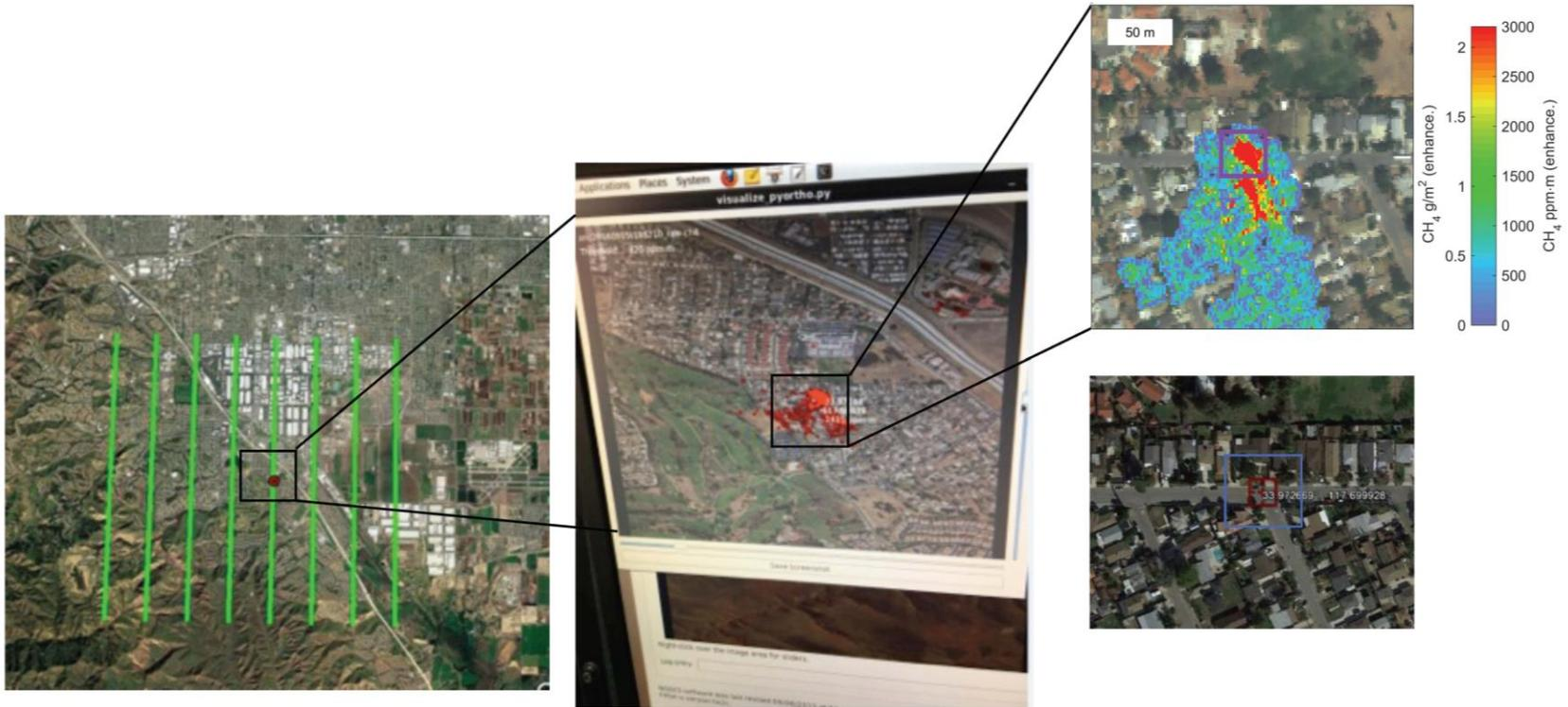
**Example of gas leak detection and repair in Chino Hills. Left: AVIRIS-NG flight pattern, middle: real-time detection software on airplane, right: processed methane plume image and geolocation of source to within 10 meters.**
