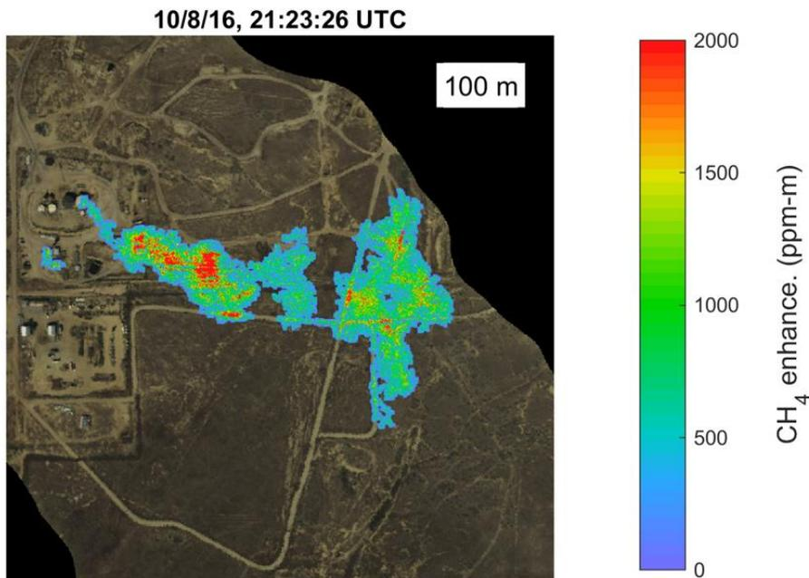
Example of a typical storage tank (from Kern Front oil field). This plume was consistently through at least September 2017 after initial detection from NASA airborne campaigns since 2014, suggesting a mechanism other than normal intermittent pressure relief valve actuation.
