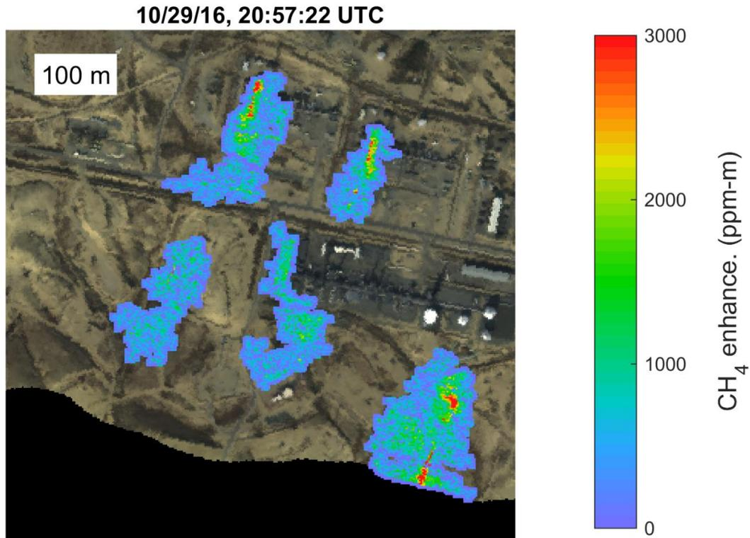
Gas processing facility in Elk Hills showing methane plumes from two of three large compressors (top) and one or more flaring stacks (bottom). These are all highly intermittent sources.
