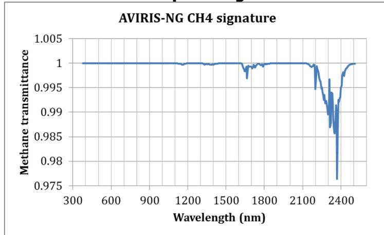
**Methane absorption signature (transmittance) plotted for the wavelength range measured by AVIRIS-NG. Strong absorptions are present between 2,200 and 2450 nm.**
