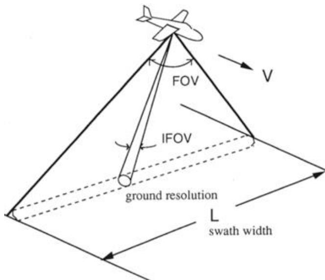
$L$ =image swath width,  $V$ =aircraft velocity, FOV=field of view, IFOV = instantaneous FOV.
