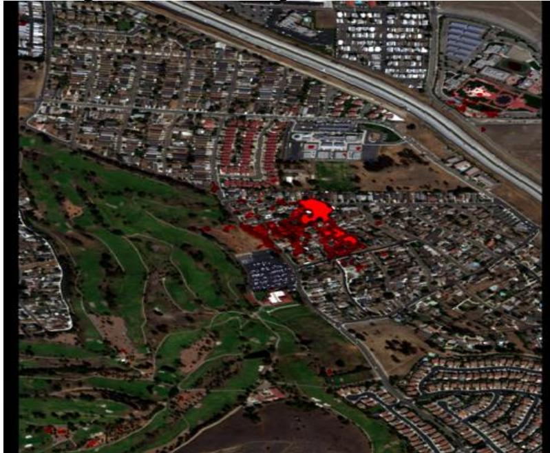
Methane quick-look products are generated at the end of each flight day. This example shows a plume from a leaking low-pressure gas pipeline that was confirmed and repaired by the gas company.
