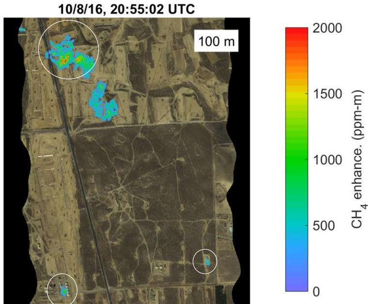
Commonly observed methane point sources in oil and gas fields include storage tanks, well heads and (potentially) gathering lines. Example shown is in Kern Front.
