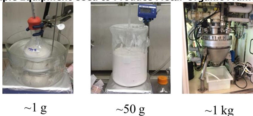
Figure 8: Sample Equipment Used to Produce Metal-Organic Framework Material
