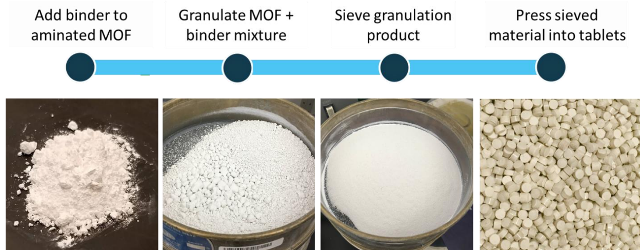
Figure 10: Steps to Convert Aminated Metal-Organic Frameworks into Tablet Form
