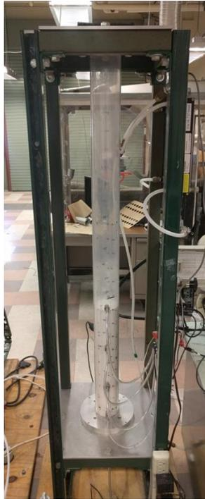
Photo of vertical fluidized bed experiment, along with four pressure probes in the fluidized bed. The cold-flow model is used to determine fluidization parameters for gasifier and methanation bed materials.
