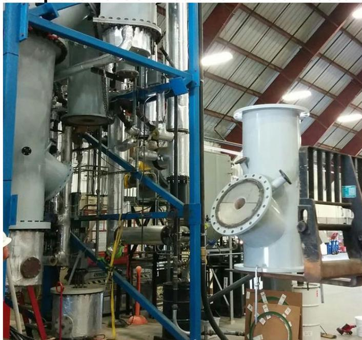
Photograph during installation of a newly repaired combustor section of the FICFB gasifier. The solid foam insulation was replaced with a poured refractory insulation, and baffle plates were welded inside the main flanges. This is to prevent gas flow near the metal walls.
