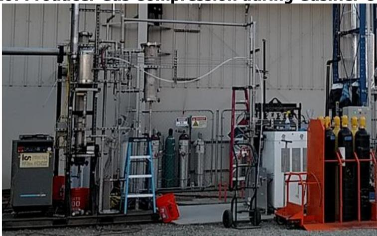
Photograph during operation of the FICFB gasifier. To the left, the chiller and chilled scrubber are shown. To the right, the compressor and producer gas cylinders are shown.
