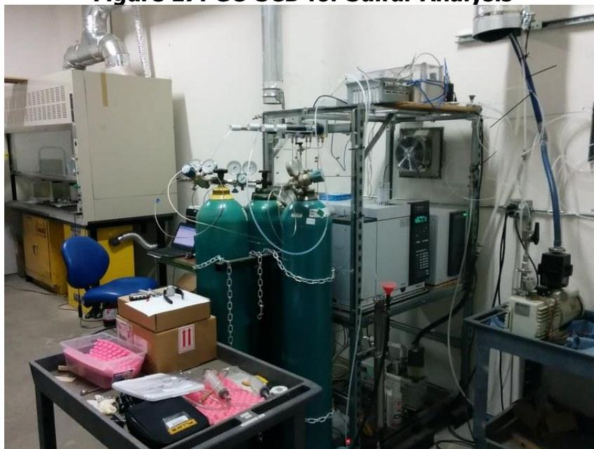
Setup for analysis of sulfur samples with a GC-SCD (gas-chromatograph with sulfur-chemiluminescence detector).
