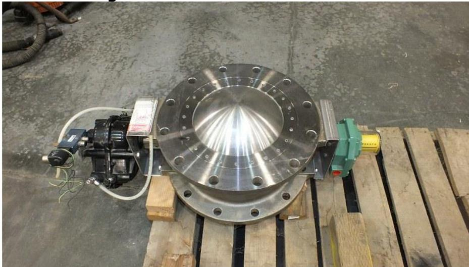
Photograph of Roto-disc valve used for the lock hopper of the biomass feeding system. The Roto-disc valve was used to replace a knife-gate valve and provided better sealing at moderate pressures. It was also less susceptible to jamming by fine feedstock particles.
