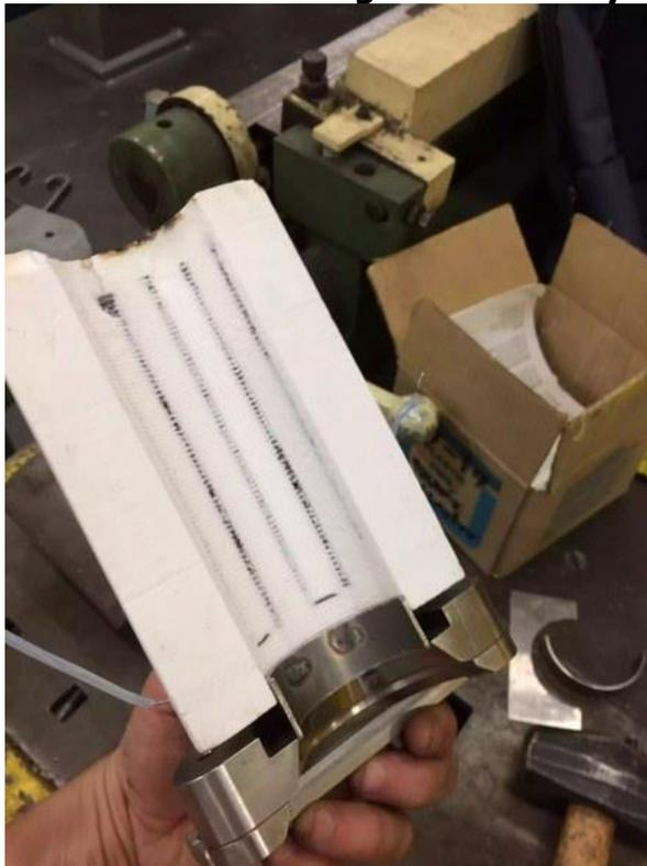
Ceramic heater for preheating of laboratory methanation reactor. The heater is mounted above the air knife that provides the cooling flow. The heater is used to preheat the reactor and to compensate for heat loss to keep the reactor at operating temperature.
