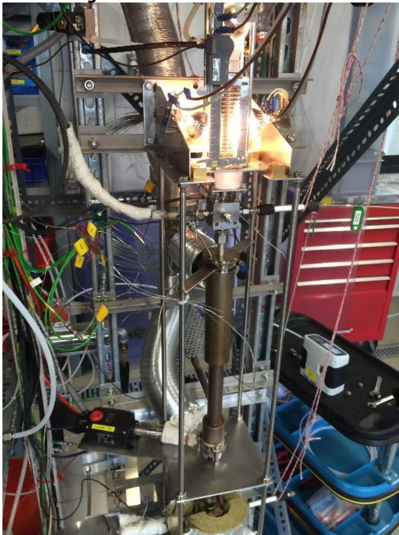
**PSI microBFB reactor with axial auto sampling system at PSI in Switzerland. The reactor has a flow rate of 1-6 slpm and is air cooled.**
