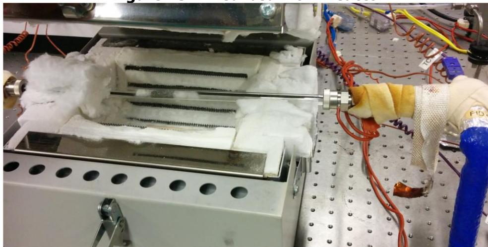
Setup for characterizing methanation catalysts in a laboratory fixed-bed reactor.
