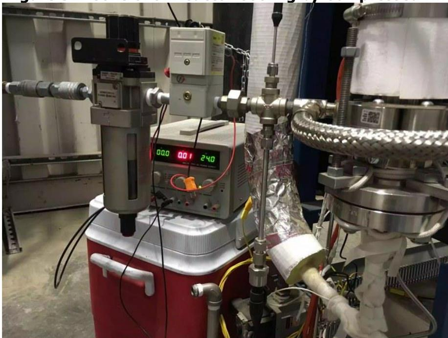
Control of reactor cooling by compressed air. Shown in the figure are a constant-pressure regulator with dryer, an electronically controlled pressure regulator, and the methanation reactor (from left to right).
