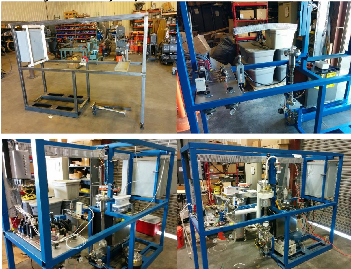
**Catalytic synthesis unit fabrication and assembly. Fabrication from 2" structural tubing with fork lift channels (top left) and assembly through time (top right, bottom left, and bottom right).**
