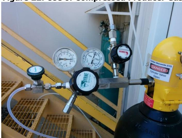
**Photo of gas cylinder with collected producer gas from gasifier test (2016/03/30) together with stainless regulator and FEP line to adsorption experiment.**
