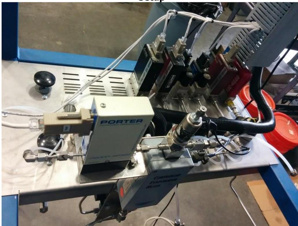
Gas and steam generation components. A micro-boiler is used to evaporate water and the system can be setup with up to 9 mass flow controllers (MFCs) for control of up to 9 gases. The picture shows 6 MFCs installed and ready for operation.
