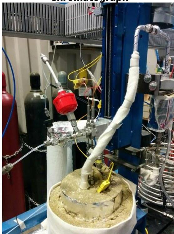
Laboratory methanation setup with gas sampling to gas-chromatograph. The red vessel contains desiccant to dry the sample before being analyzed by the gas chromatograph. The insulated part shows the top of the methanation reactor.
