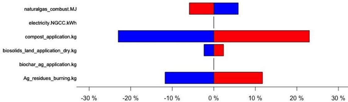
The y-axis represents percent change in net lifecycle GHG emissions for a given scenario due to a change in a specified parameter or process. The red bars represent positive changes and the blue bars represent negative changes as explained in Table 43.
