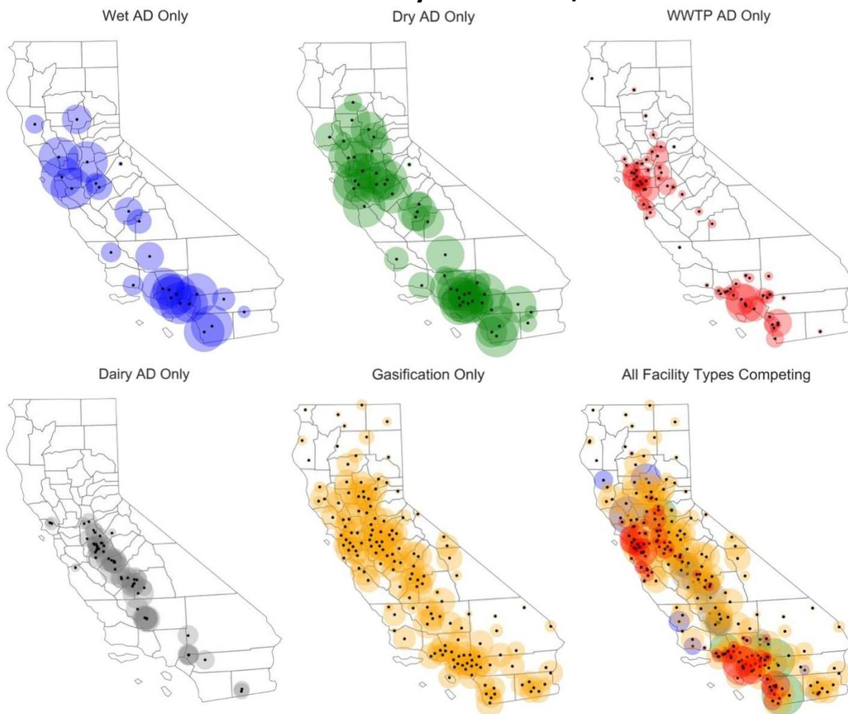
**Red = WWTP co-digestion facility; green = dry AD facility; blue = wet AD facility; grey = dairy AD facility; yellow = gasification facility. Size of circle represents relative quantity of waste intake.**
