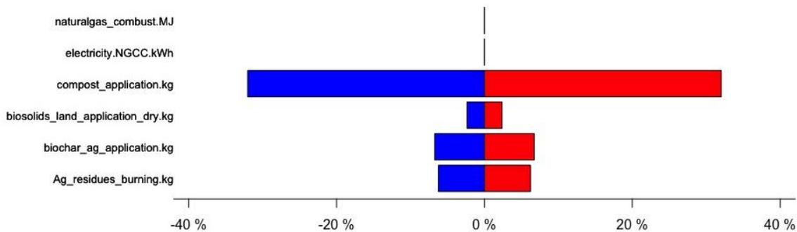
The y-axis represents percent change in net lifecycle GHG emissions for a given scenario due to a change in a specified parameter or process. The red bars represent positive changes and the blue bars represent negative changes as explained in Table 43.
