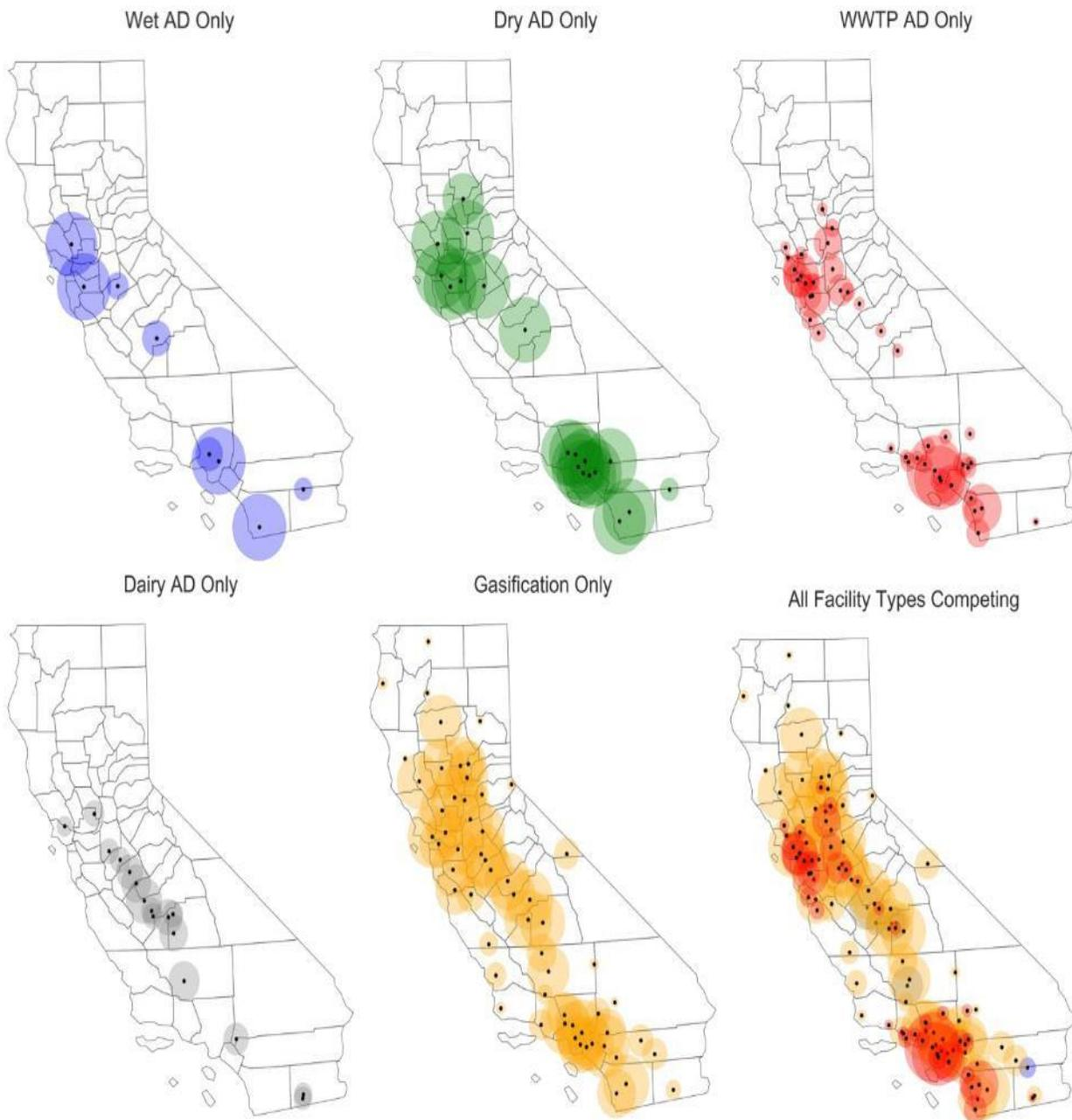
**Red = WWTP co-digestion facility; green = dry AD facility; blue = wet AD facility; grey = dairy AD facility; yellow = gasification facility. Size of circle represents relative quantity of waste intake.**
