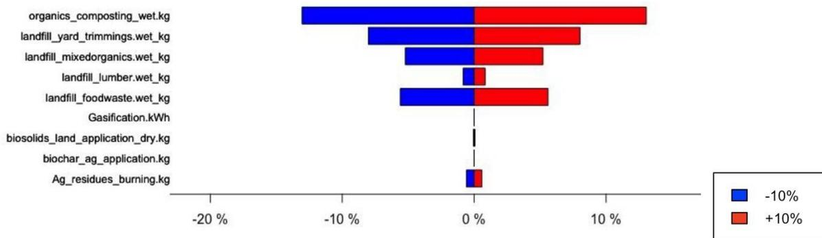
The y-axis represents percent change in net lifecycle GHG emissions for a given scenario due to a change in a specified parameter or process (as indicated by the legend).
