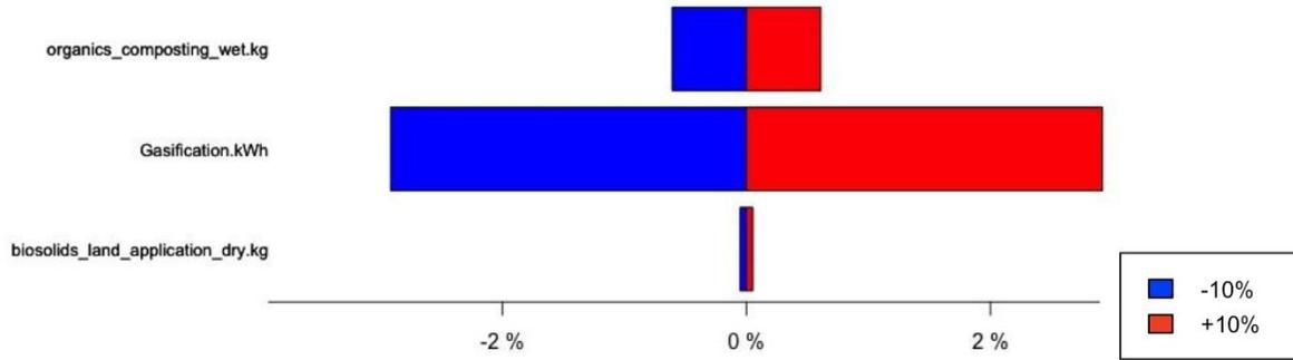
The y-axis represents percent change in net lifecycle GHG emissions for a given scenario due to a change in a specified parameter or process (as indicated by the legend).
