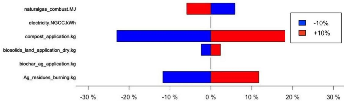
The y-axis represents percent change in net lifecycle GHG emissions for a given scenario due to a change in a specified parameter or process (as indicated by the legend).
