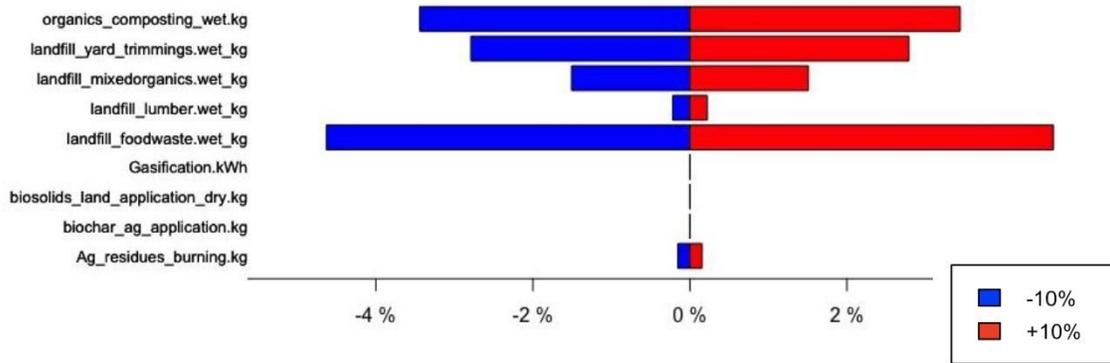
The y-axis represents percent change in net lifecycle GHG emissions for a given scenario due to a change in a specified parameter or process (as indicated by the legend).
