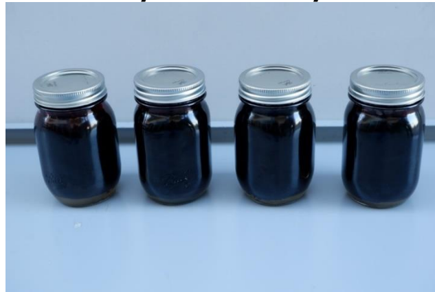
Figure 17: Output of Biocrude inside of Containerized Hydrothermal Processing System at Factory
