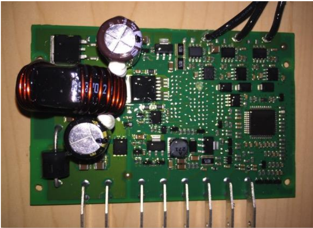
Figure 32: Danfoss/Secop Inverter Board
