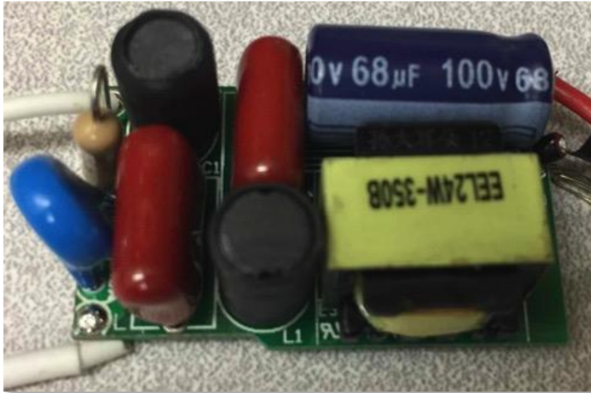
Figure 39: Original Alternative Current Light-Emitting Diode Driver
