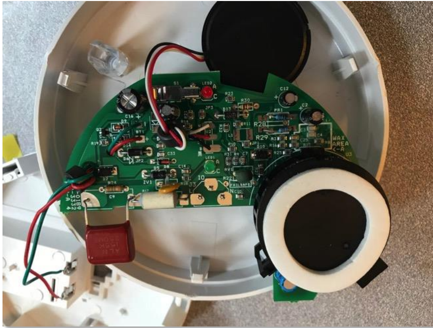
Figure 60: Teardown of the SMA36 Smoke Alarm—Electric Circuit
