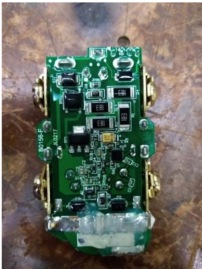
Figure 59: GFO17 GFCI Outlet Teardown—Electrical Circuit
