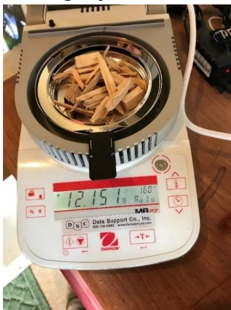
Figure 21: Testing Dry Fuel for Moisture Content
