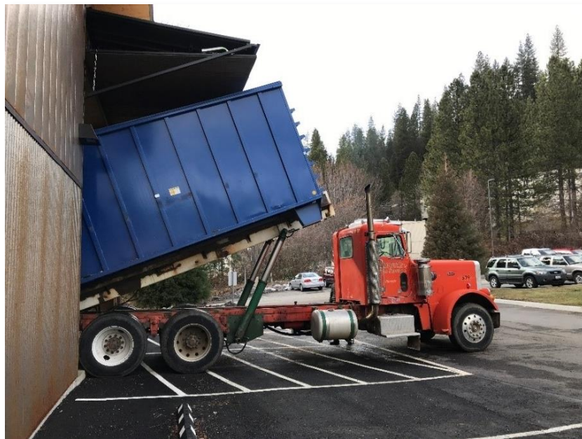
Figure 6: Roll-Off Truck Returns Full Bin to Boiler Building
