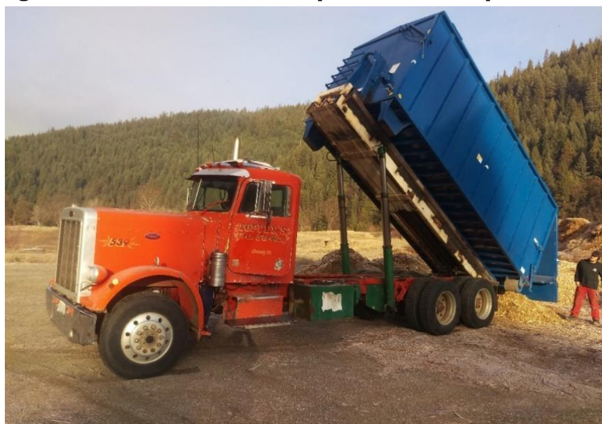
Figure 13: Roll-Off Truck Empties Wood Chips from Bins
