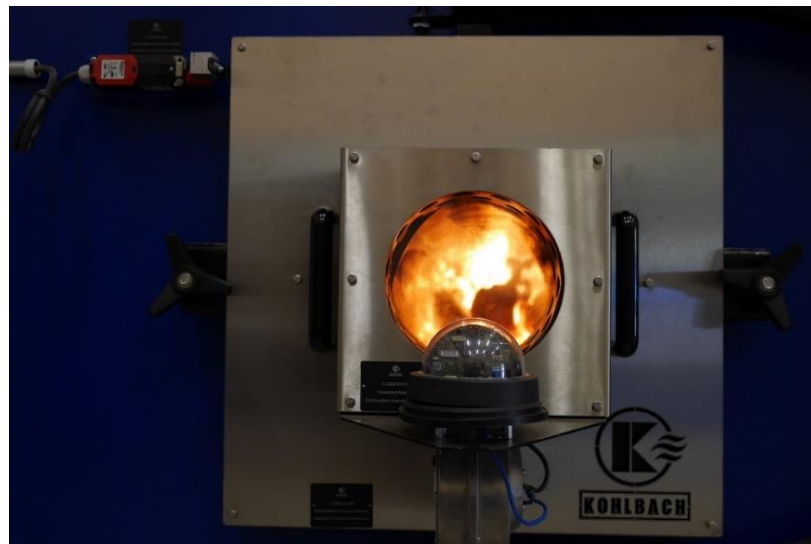
Figure 2: Observation Portal to Combustion Chamber
