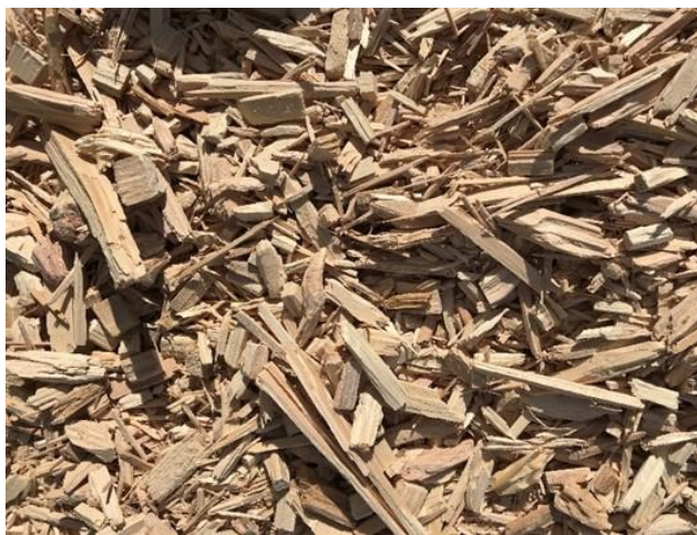
Figure 20: Dry Fuel, Ideal Feedstock for Efficient Boiler Operation
