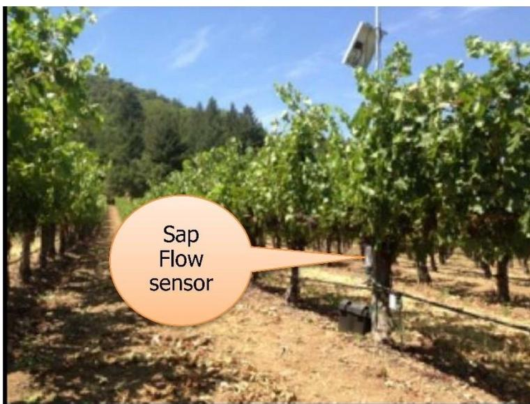
**Grape vine equipped with a sap flow sensor.**
