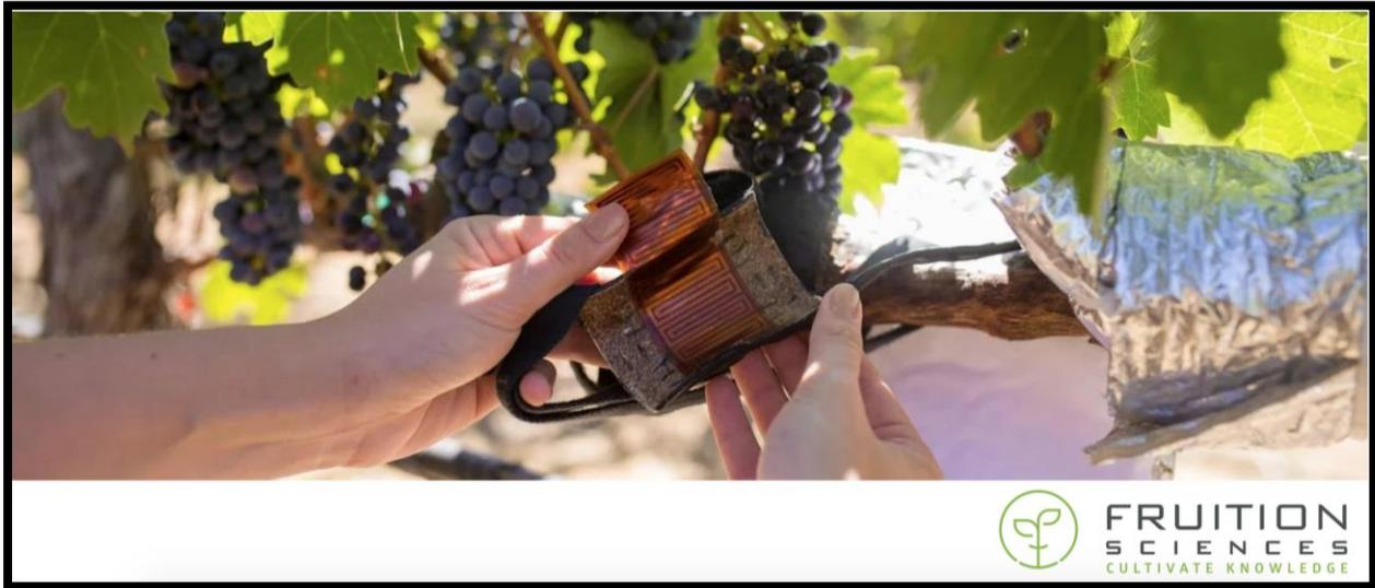
**Picture shows the inside of the sap flow sensor. Orange sleeve applies heat around the stem. Thermocouples are embedded with the cork material for heat displacement measurement.**
