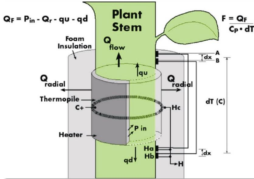
Picture shows heat fluxes measured inside the sap flow sensor.
