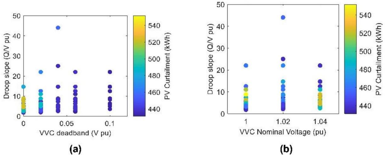
(a) volt-var control deadband and (b) volt-var control nominal voltage. Total uncurtailed PV generation ranges between 2,348 – 65,503 kWh per day for all PV days and increased hosting capacities on all locations. The curtailment in the figure corresponds to 5.2 – 6.1 percent of total PV generation on the corresponding PV day/location.
