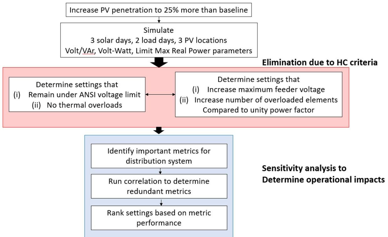
**Flowchart describing the process of determining which settings should be recommended for Phase 3 smart inverter functions.**
