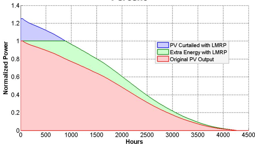
**Notes:** PV power is normalized to the original AC rating. With the LMRP function set to 80 percent, the new system size is 25 percent higher than the original, yet the power output never exceeds the original peak value (shown at the height of the green area). While there is some curtailed energy (blue area), the increased size allows for more total energy (green area) than the original PV size (red area).
