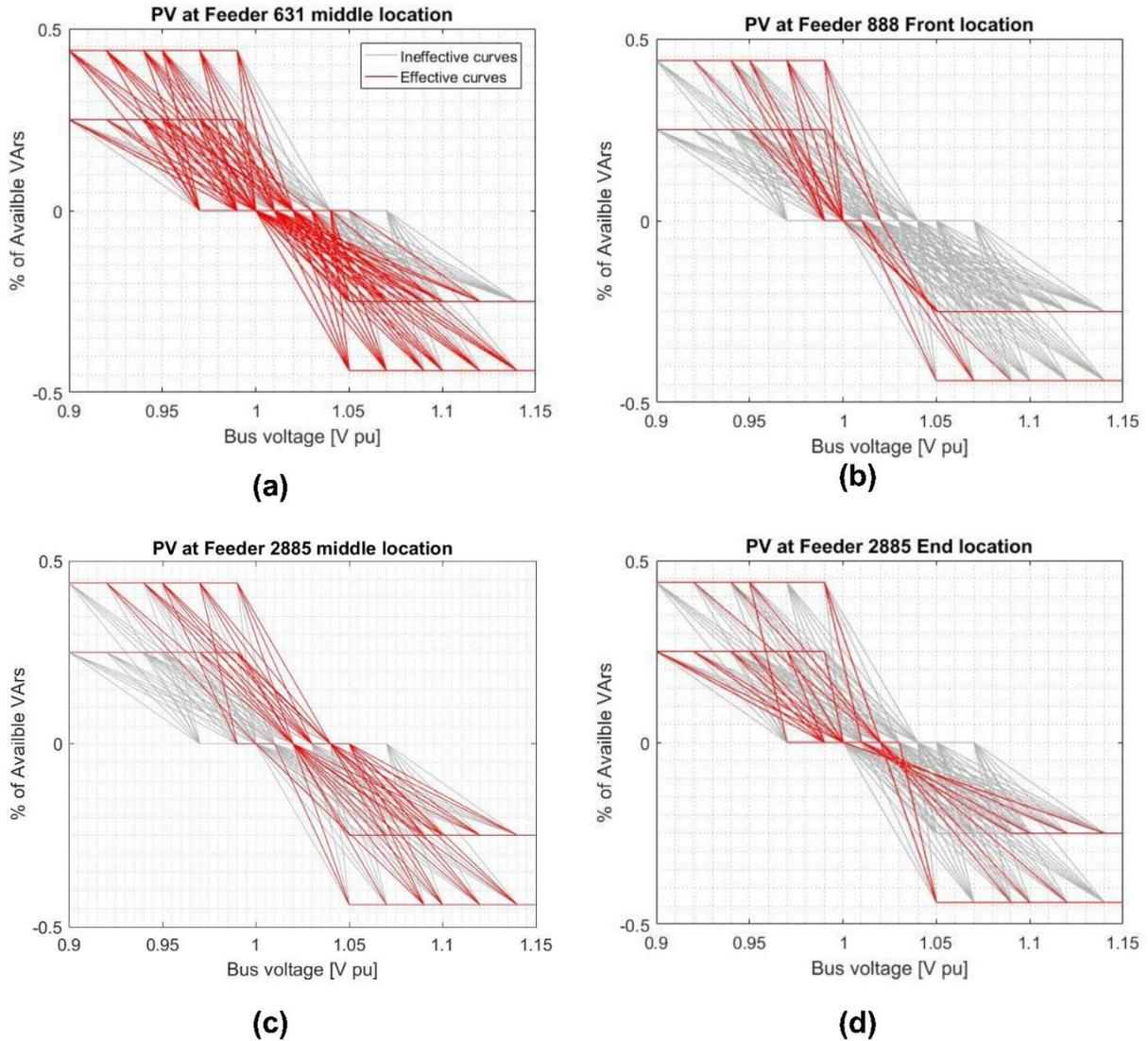
**(a) Feeder 631 – PV at feeder middle, (b) Feeder 888 – PV at feeder front, (c) Feeder 2885 – PV at feeder middle, (d) Feeder 2885 – PV at feeder end.**
