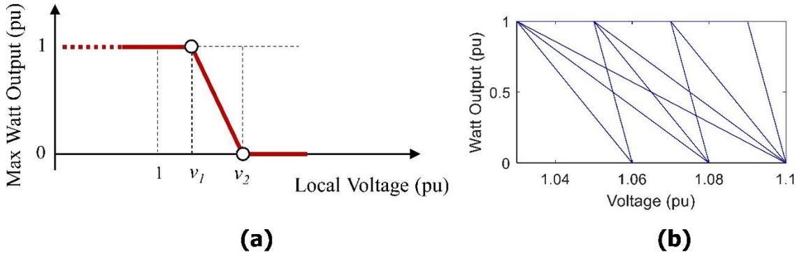
(a) Settings curve of volt-watt function [18]. The deadband starts at 1 V pu and ends at  $v_1$ , and the watt output is curtailed based on the steepness of the droop slope past  $v_1$ . (b) The analyzed volt-watt settings (nine curves) extend beyond the lowest and highest voltage points shown in the figure.
