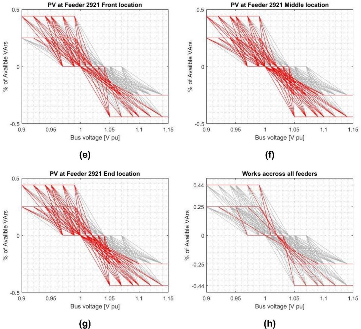
**(e) Feeder 2921 – PV at feeder front, (f) Feeder 2921 – PV at feeder middle, (g) Feeder 2921 – PV at feeder end, and (h) the 13 curves that work for all seven scenarios plotted in (a–g). Other feeders/locations are excluded since there are no voltage violations.**
