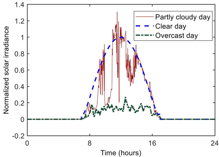
**Three representative solar days from the time series, clear, partly cloudy, and overcast. All-time series are normalized to the peak irradiance on the clear day.**
