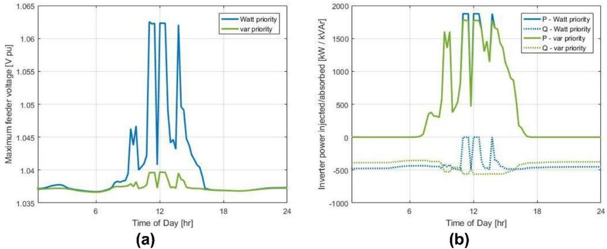
**Comparison of watt and var priority for setting 180 on Feeder 2921 when the PV source is at the end of the feeder for the partly cloudy day with minimum feeder loading. (a) Voltage time series. (b) Active and reactive power output from the inverter.**
