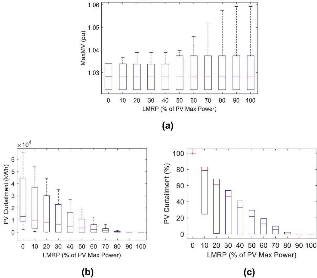
**(a) Maximum MV vs. LMRP settings. Curtailed PV generation in (b) kWh and (c) percent curtailed vs. LMRP settings.**
