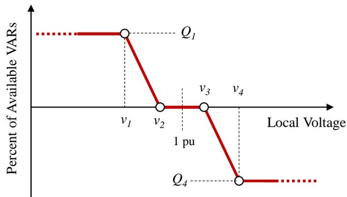
**Volt-var curve using available reactive power of PV system to control voltage. Values of  $v_1, v_2, v_3, v_4, Q_1$ , and  $Q_4$  are modified as shown in Figure 8 [17].**
