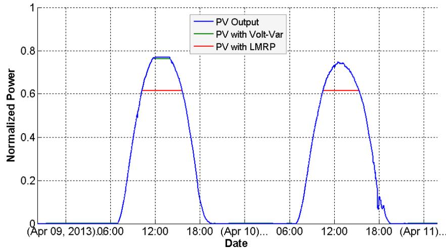
**Notes: PV power is normalized to the DC rating. Given that the DC/AC ratio is 1.3, the maximum power output relative to the DC rating is 76.9 percent; thus, the maximum curtailment from the volt-var function is 76.9 percent × 96.8 percent = 74.5 percent.**
