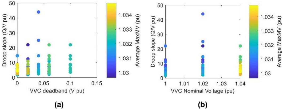
Average over 18 solar load PV location days. (a) volt-var control deadband and (b) volt-var control nominal voltage.
