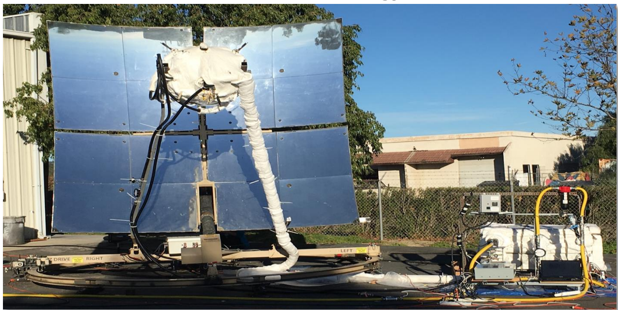
Figure 53: Final CSP-TES Assembly Used for the On-Sun Demonstration of the SulfurTES Technology
