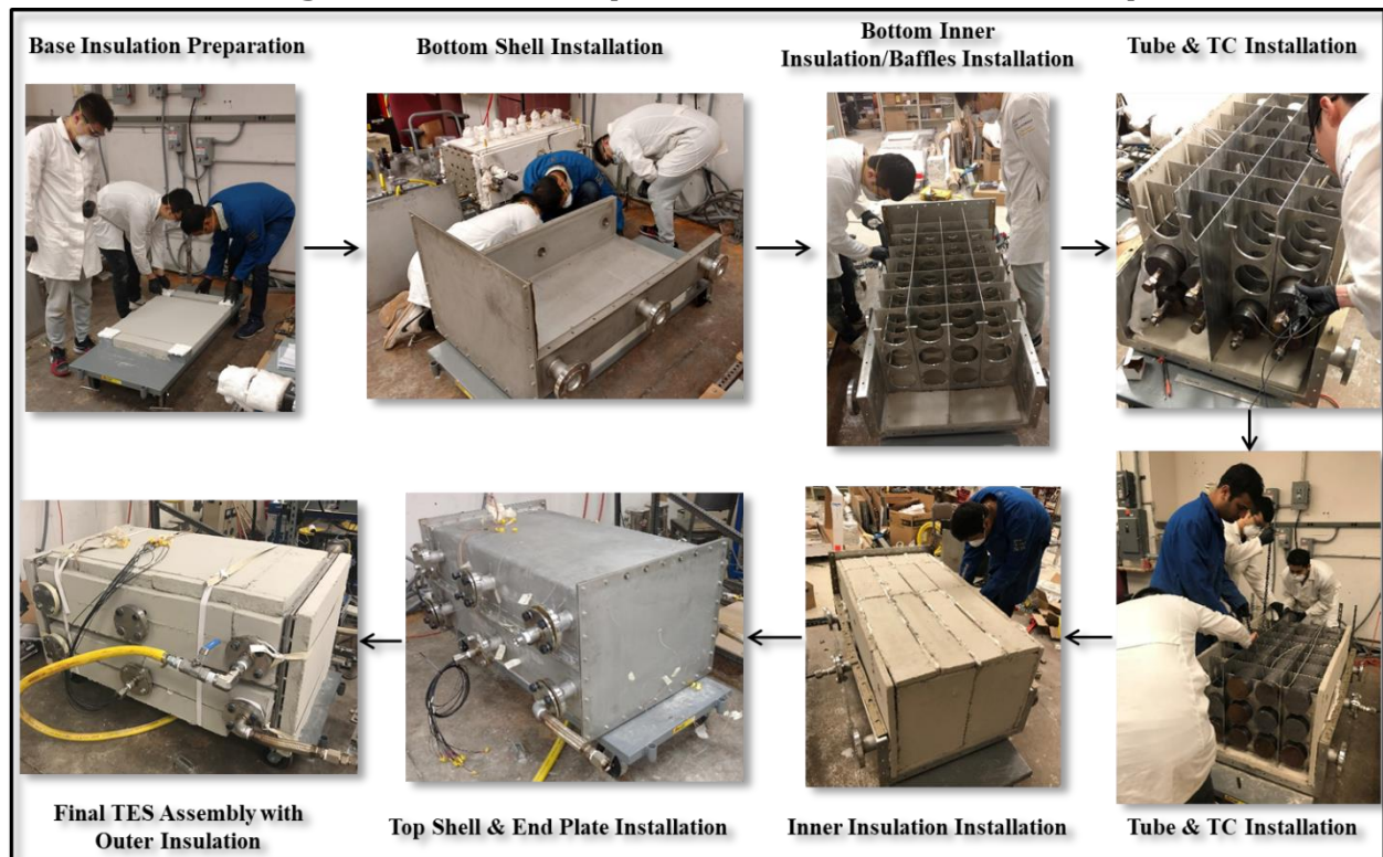
Figure 47: Assembly of 30 kWh SulfurTES Battery
