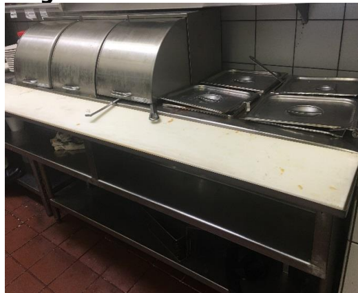
Figure 267: Right Steam Table with Dual Bulb Burners
