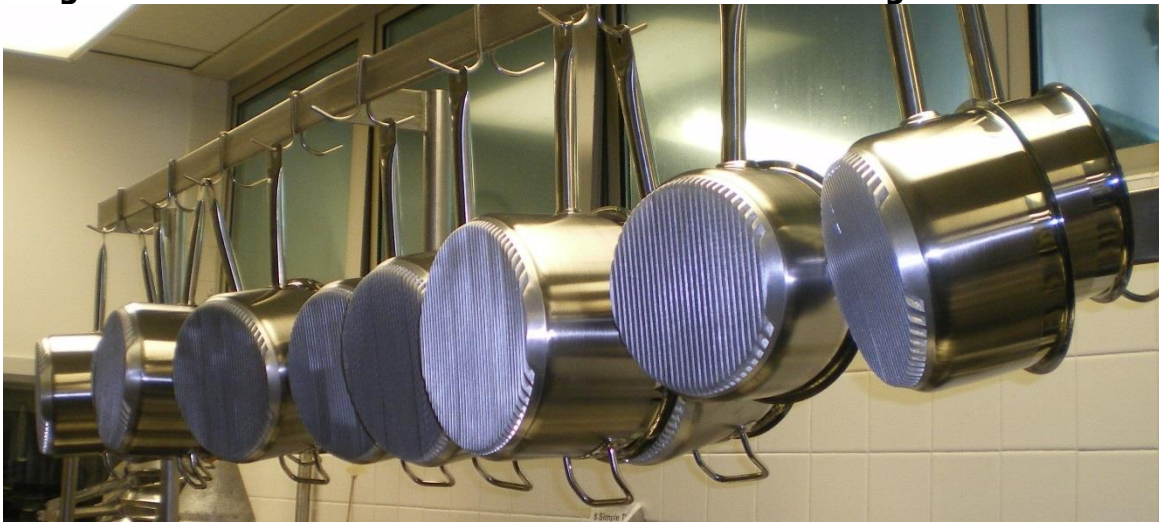
Figure 189: Finned Bottom Pots for Increased Cooking Heat Transfer
