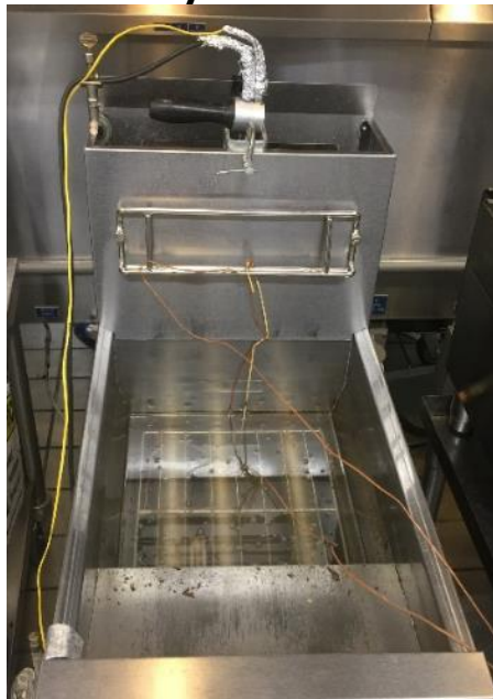
Figure 297: Fryer Flue Measurement
