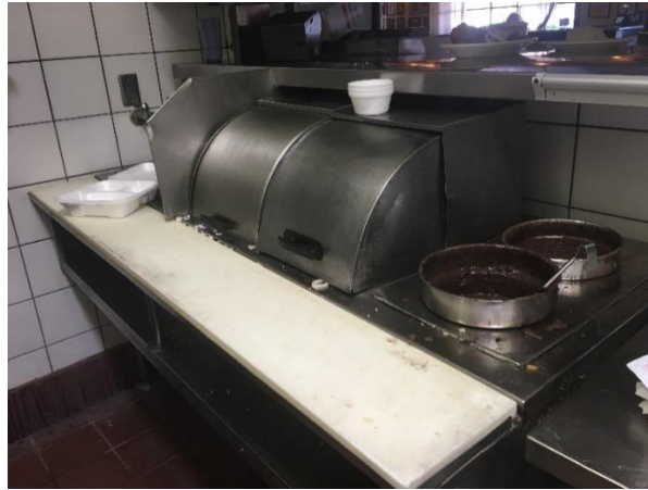
Figure 266: Left Steam Table with Tube Burner
