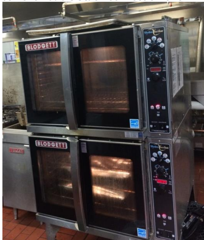
Figure 145: Replacement Double Stack Convection Oven with Steam Injection
