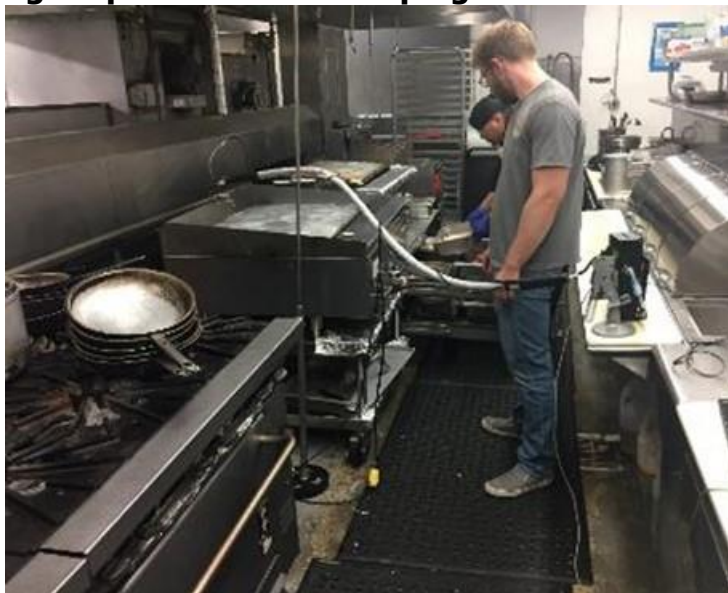
Figure 341: Manifold sampling probe was placed in the high O 2 sampling zone region to mitigate potential flame impingement as observed in the lab
