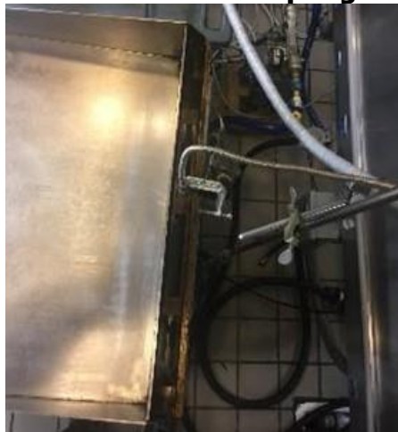
Figure 325: Lab set up with a top view of the griddle and the manifold probe positioned in the sampling zone
