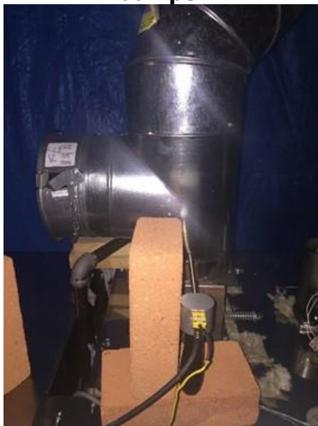
Figure 330: Hole was drilled to fit the probe into a closed duct below the flue damper
