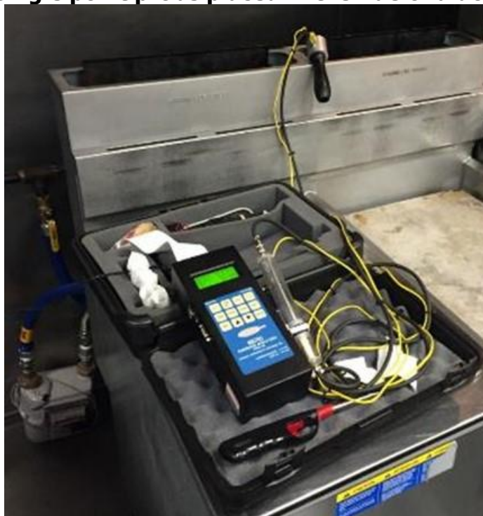
Figure 342: Single point probe placed in the flue of a double vat fryer
