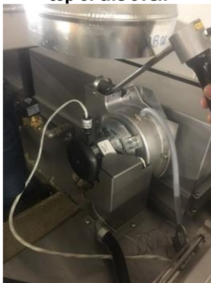
Figure 329: Emissions sample was taken at the outlet of the blower exhaust fan on top of the oven
