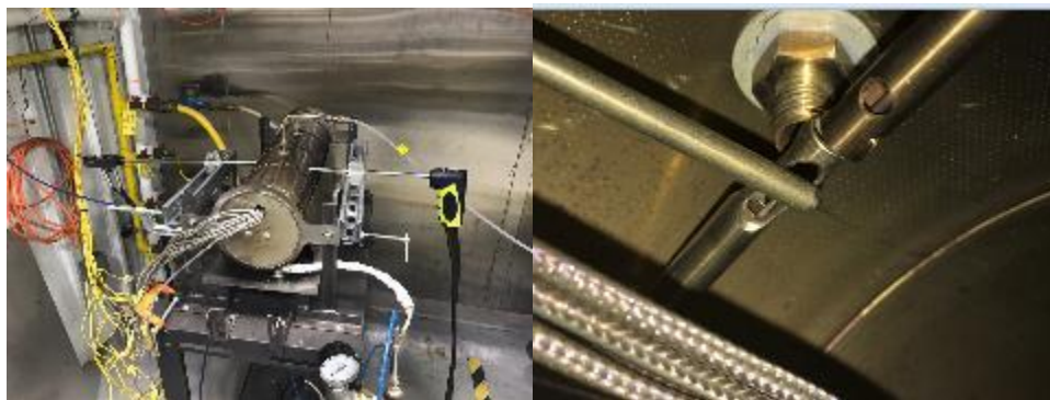
Figure 334: Tube Burner Test Setup and Different Emissions Probes inside of Test Stand
