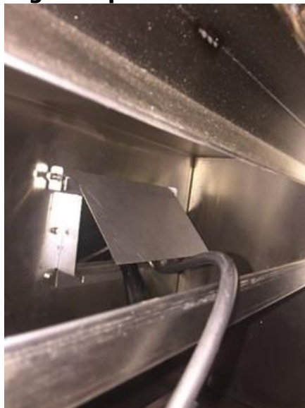
Figure 331: Direct-fired rack oven combustion products are exhausted from an opening on top oriented to the front
