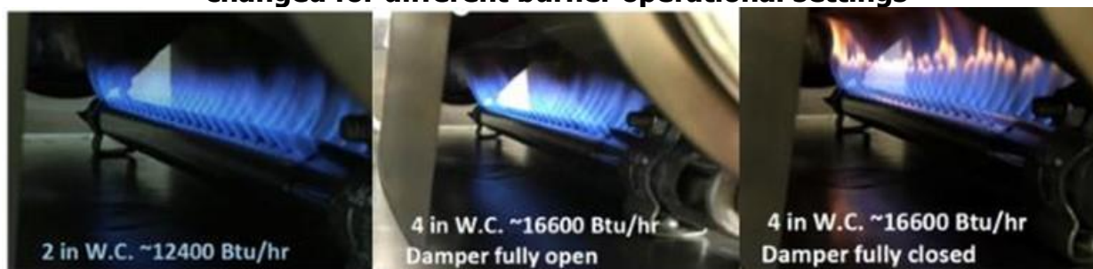
Figure 335: Tube Burner Test at Different Test Conditions: appearance of the flame changed for different burner operational settings
