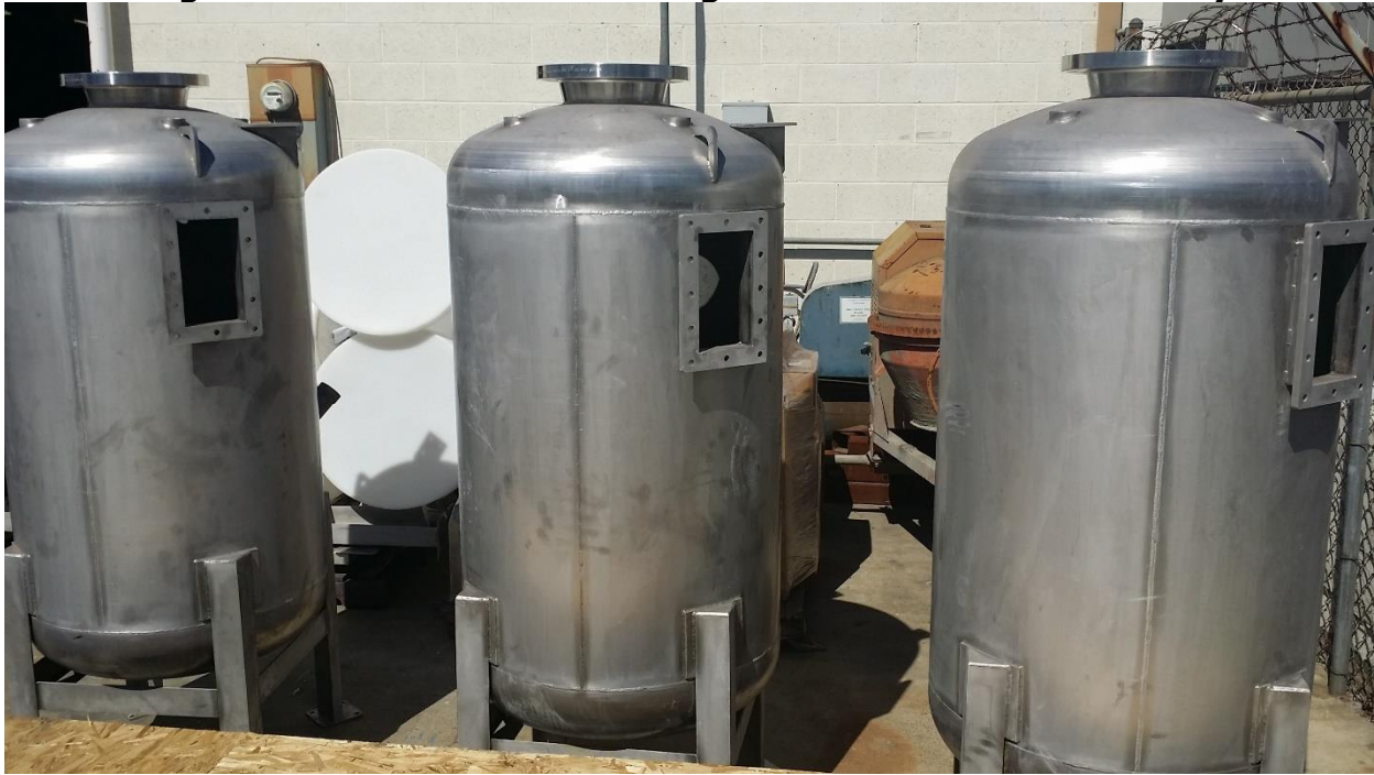
Figure 3: 316 Stainless Steel Digester Tanks Before Assembly
