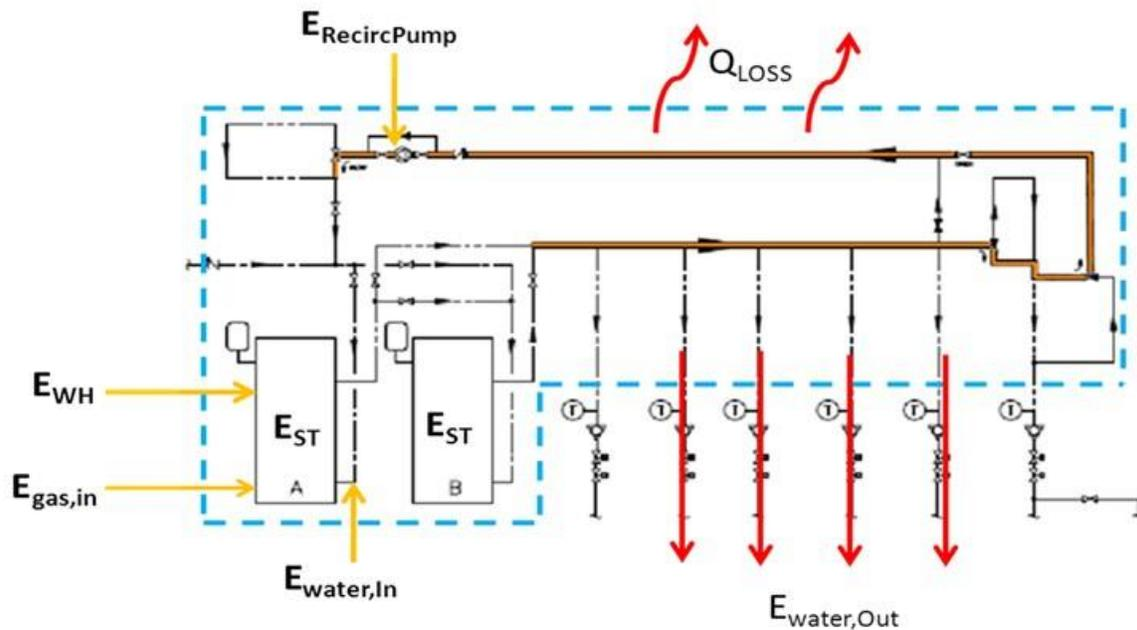
Energy storage only taken into account when testing storage heaters.
