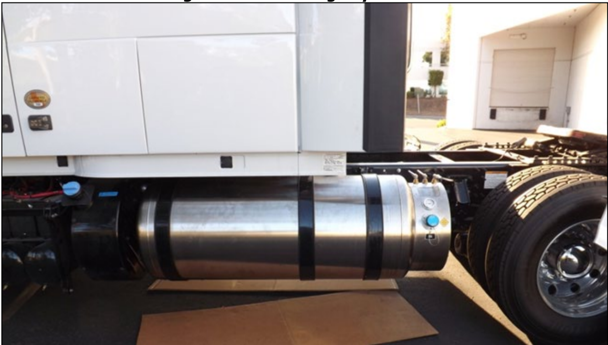
Figure 7: LNG Storage System
